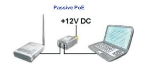
You don't want to power ALF with 24V DC because you have in your network PoE "Power over Ethernet" in use. No problem, ALS provides passive PoE, this means he can be powered with the not used cables of the lan-cable with 12V DC. You don't need additional the 24V DC. **Attention:**Don't connect a PoE-cable to a lan-client which don't provides PoE! The device could be damaged!
