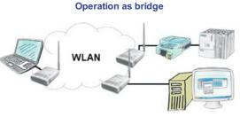
You have two or more clients which should communicate together without LAN-cable-connection? No problem, you connect a "Access-Point" configured ALF to this device and to the other device a "Client" configured ALF. Then connect the "Client" with the "Access-Point" and the device are able to communicate together.
