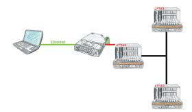
With the S5-H1-PG-LAN you would be able to use the H1-path-selection over the S5-LAN++ and communicate with all PLCs in the H1-bus. You don't have to connect serial to the CP, you can do this easy over your network.
