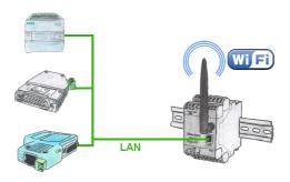
You also need to network devices but dont have locally no ethernet-cable. Wifi is available? With the EtherSens-Bridge you bring immediately all connected wired participants in the WLAN network.
