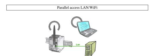
Access parallel via LAN and Wifi to the EtherSens-device. Therefor create via the web-server for each way an ip-address, regardless whether its the same subnet or not.
