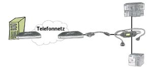
You have to reach urgend your PLC via remote maintenance and have no TS-adaptor in your company? No problem, configure with the MPI-Kabelmanager your S7-interface-cable MPI-II-Kabel the mode "TS" for "remote maintenance", connect this cable with the TS-Adapter (article number 9350-TS) with a standard modem and send it all to your client. Now you will be able to start the connection with your TS-sofware and solve the problem. And this all without buying a original TS-adapter.
