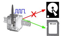
With the integrated SD-card-slot you back-up the recorded data in the device and dont need an external memory. Nevertheless you can send additional the data via FTP to a FTP-server.
