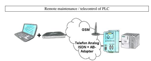
The access to the connected PLC with the Siemens TS-software or PG-2000 including TS-option results of coupling via Analogue-, ISDN- (only with AB-adapter) as well as GSM-line.
