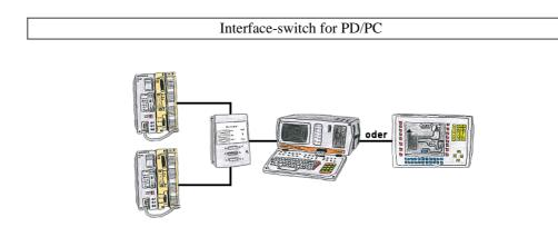
You have to work with more PLC-devices, but no pleasure to switch on/off? No problem, you connect a device of the AG-Switch-family to the PLC-devices and your PD/PC and you will be able to communicate to both PLCs. The selection which PLC you make for AG-Switch-I via toggle switch and for the AG-Switch-II via 24V-controll input.
