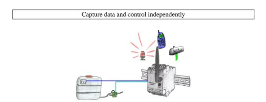
Apply small control tasks of your systems with EtherSens-Control-devices. Determine switching points where the device is running to respond. Depending on the parameterization, an email or SMS notification (depending on the device-configuration) or the device automatically controls via the optional IO-modules (analog / digital / relay).
