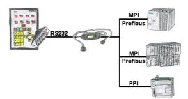
Your panel provides a serial port and no MPI/Profibus for connecting a S7-PLC. Connect the MPI-II-cable with it and you're Online with your panel.
