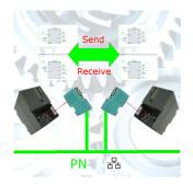
Coupling S7-controller with MPI/Profibus at S7-controller with MPI/Profibus via network
