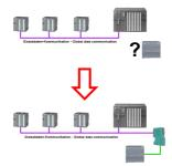
Running global-data-communication between MPI-PLCs (S7-300/400), is one of these PLCs replaced with a newer PLC with network-interface (S7-1200/1500), this PLC was not able to access this data.
