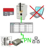
S5-PLC triggered DB-backup/-restore without additional PC via PG-socket and Ethernet on SD-card
