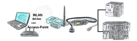
Your're right in the middle of your production line and and should move around the machine and simultaneously observe / manage. No problem, you parameterize the S7-WLAN-Bridge, connect to the MPI-LAN and connect to an access-point or with the ad-hoc-network of your laptop and are ONLINE on the PLC.
