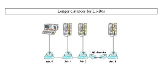
You need for your L1-Bus higher distance like the possible 1200m? You have strong distrubance on your L1-Bus? You need a serial line for higher distances and this galvanic decoupled? No problem, all this points are solved through the LWL-adapter. They are available for artificial and optical fibre, for L1-Bus and RS232.
