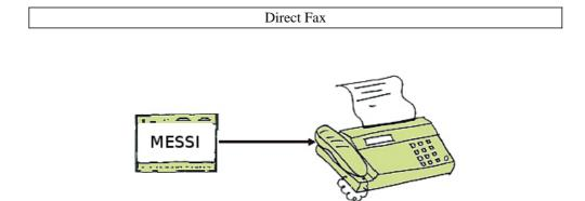
By direct dialling up the fax machine a message is carried out to a fax-receiver. If a connection comes off the message will be transmitted.
