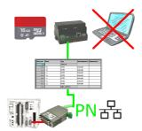
S5-PLC triggered DB-backup/-restore without additional PC via PG-socket and Ethernet on SD-card
