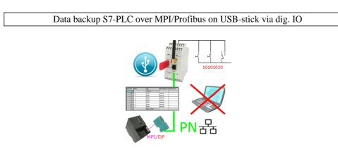
Via digital input triggered DB-backup/-restore without additional PC via MPI/Profibus to USB-stick
