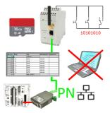
Via digital input triggered DB-backup/-restore without additional PC via PG-socket and Ethernet to SD-card
