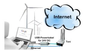
You are on site at your plant, right in the field and have no electrical outlet in order to realize your internet-access by Toni. Plug the USB-powercable into a free USB-port on your PC, connect it to the Toni and you will have immediate access to the internet.
