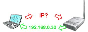
You use your PC in your company network with DHCP, so you dont have to care the everlasting setting of the ip-address. No problem, ALF also can be configured as a DHCP-server and assigns you accessing to the device via LAN or WLAN an ip-address from a predefined address range.
