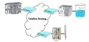
Your pumping stations report the water levels of the central control via telephone network. The central office itself can of course transmit commands/messages to the substations as well. Thereto no dedicated line is required, a "normal" telephone connection is sufficient because the devices hangs up the line after occured message.
