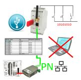
Via digital input triggered DB-backup/-restore without additional PC via PG-socket and Ethernet to USB-stick
