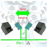
Coupling S7-controller with MPI/Profibus at S7-controller with MPI/Profibus via network
