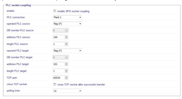
The following parameters are available for the PLC socket coupling:
