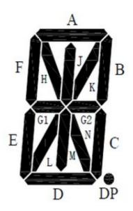
To switch segments on or off you always have to write the complete value of the letter. Every segment is represented as a single bit within a 16 bit value (most significant bit is always 0). The structure of the value is as follows:
