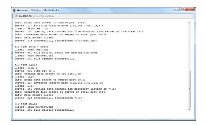
With the help of the connection test you can test the connection and detect errors in your configuration. At the connection test many of the FTP commands that are used by the EtherSens are used. Beside the basic commands *USER*, *PASS*, *CWD*, *TYPE*, *PORT*, *PASV* and *QUIT* EtherSens is using the commands *RNFR*, *RNTO*, *DELE*, *SIZE*, *STOR*, *APPE*, *RETR*, *LIST* and *ABOR* for the data transfer and connection control.
