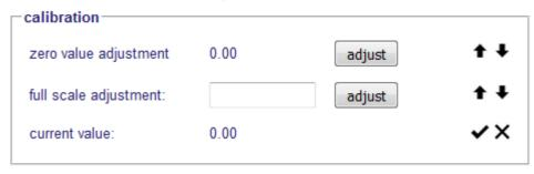
With the help of the (general) calibration pop up you can executed a zero point and full scale adjustment. The resulting offset and the gradient is calculated automatically, stored in the configuration and used for calculating the viewed value.
