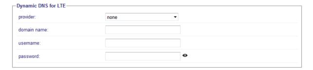
For configuring the DDNS service (Dynamic DNS) for the LTE module the following settings are available:
