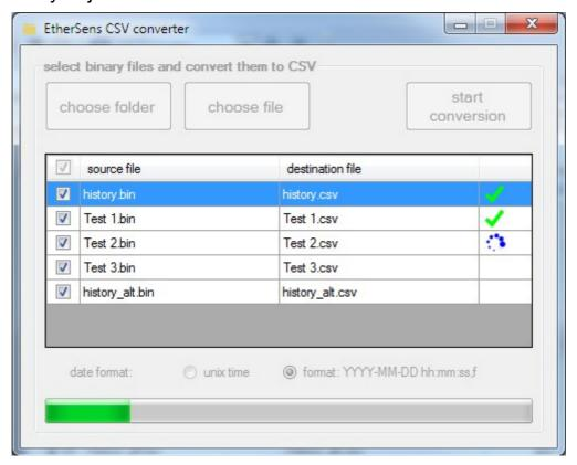
The icon on the last column of every entry shows the state of the conversion. The progress bar shows the progress of the current file.
