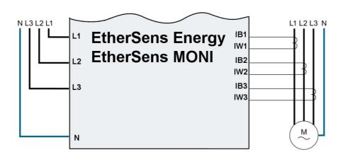
Of course you can only connect L1 and N (power supply for the device itself) but connect all three sensors for the current measurement. In this operating mode the power and energy can't be calculated correctly because the voltage for L2 and L3 are missing. The captures for the currents are working, because they are independent of the voltage.
