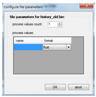
For each file which has a valid format the application will check if a .nam file for the corresponding .bin or .bak file is available. These files are stored on the SD card for a combined history additionally, if the setting "name file" on the web server in the menu item system  $\rightarrow$  storage is enabled, and contain the names of the recorded process values.
