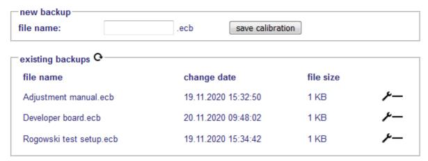
On the upper part of the dialog you store the actual calibration from the current values of the device. Therefore you have to enter a unique name into the text field and click on the button "save calibration". Afterwards a
