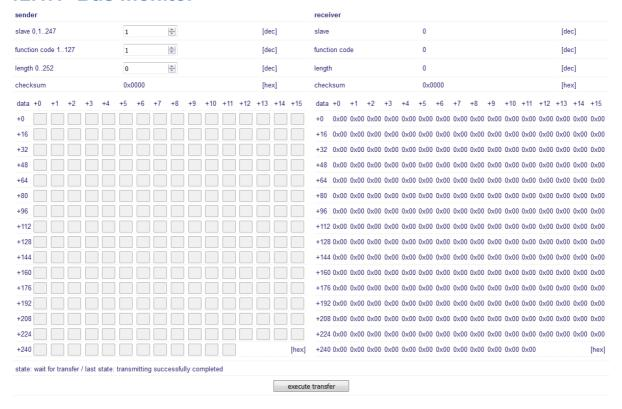
The bus monitor is the easiest way to manually send Mobus requests (e. g. to check the raw response of a slave). The monitor can be found on the page "system status" in the group "network applications". If you want to open the monitor you just have to click on the "open monitor" button in
