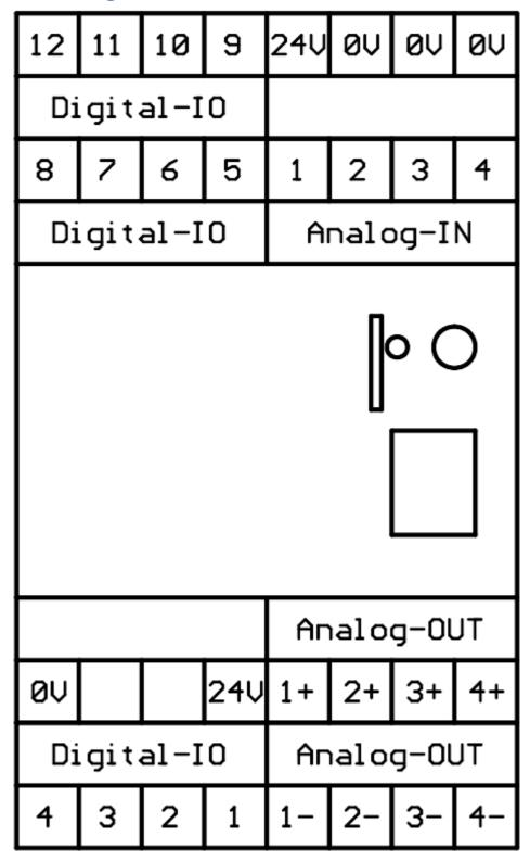
17.3.2 Port assignment EtherSens Control HW 1.1
