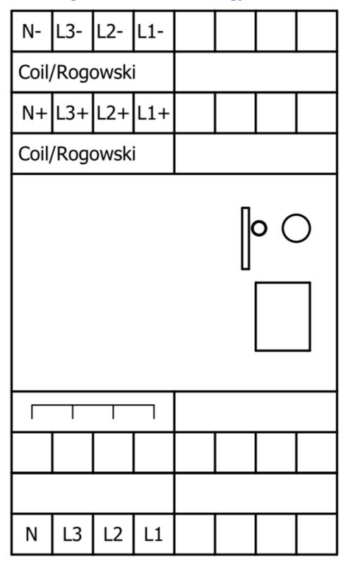
17.2.2 Port assignment EtherSens Energy + Analog-IO
