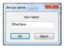
In the window you can type in the "new" name for the device. After clicking the "OK" button the name will be sent to the device and stored in the configuration.
