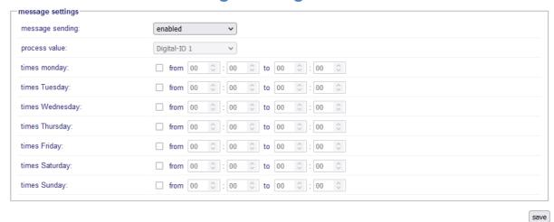
In this menu item you can configure when your device is allowed to send messages (via e-mail or SMS) which were triggered by a limit value or a recognized PLC message. With the selection list "message sending" you can choose one of the following modes:
