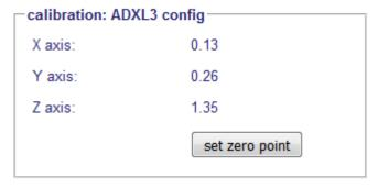
If you want to calibrate an accelerometer (ADXL3xx) you have to find the configuration process value (default name "ADXL3 config") and click on the calibration symbol in the process list.
