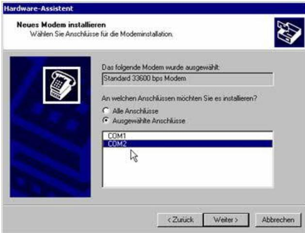
Select interface on the PC with which the Event-modem is connected to.
