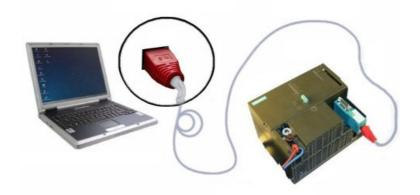
Before you can use the device you have to connect it properly. In the first step you should put your device on the MPI/Profibus interface of your PLC. If a bus cable is already connected to the interface of your PLC you can simply connect your device on top of the cable if a diagnostic jack is available. Alternatively you can also put your device on a slave module (e. g. a panel).
