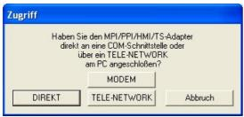
For access query choose "Direct" if your product connects via USB-cable or Nullmodem-cable. "Modem" if your product connects via telephone line or "TELE-Network" if your product connects with a TELE-Network device via telephone line.
