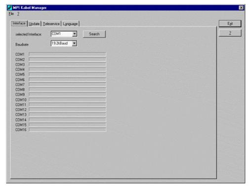
In "set interface" you can choose the COM-port you device is connected at. Only the COM-port which was aktive at starting the MPI-Kabel-Manager are shown.
