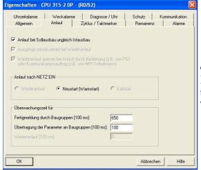
10. In your networkconfiguration you can open the objectconfiguration of your cpu.
