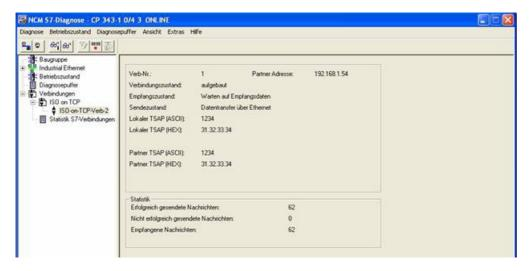
4. For added control, you can now take the DB10 in your S7 - SPS (with CP) and take the DB14 in your S7 - SPS (with S7 - LAN gateway), and check if the values of the 20 bytes you have configure in the each other PLC in DB10 and DB14 from DW0, match with those from DW100. If that is the case, the communication between S7 and S7-CP-LAN was completed successfully.
