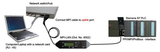
MPI-LAN Connection possibilities with operator panel
