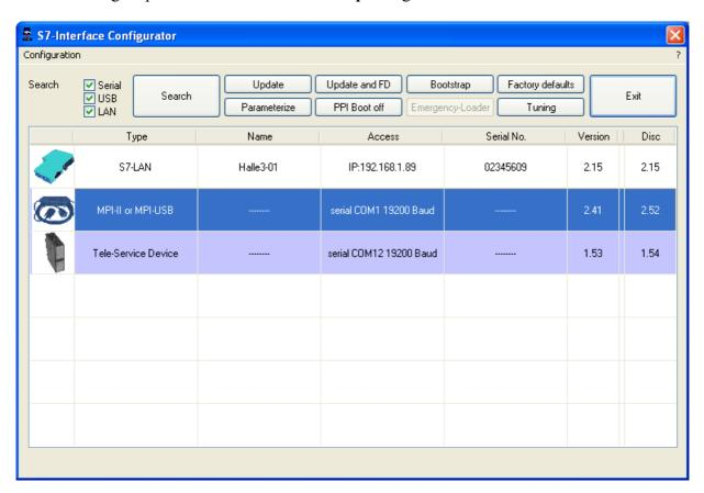
Below the buttons is a list of the found devices. In each line an image, the type of the device, name (if existing), interface, serial number (if possible) and the OS-version of the device is displayed. On the rightmost position the actual OS-version on the harddisk is displayed.
