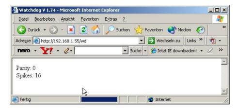
This side will refresh every second after completely loaded. The Counters are always reset to 0 when read.
