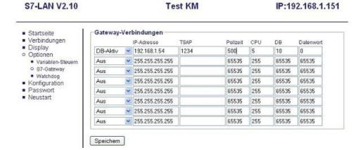
The final step is to configure the gateway. Here you have to set "Connection Type" to "DB - active" and at (the partner device" passive) "Station Number" you must enter the number of your PLC. Now you should decide which is the configuration data block in your PLC and from which data word. The IP - address of your S5 - LAN type in "IP - address partner" field. In "TSAP" you store now have the same name as in the S5 - LAN Manager your S5 - LAN are assigned.
