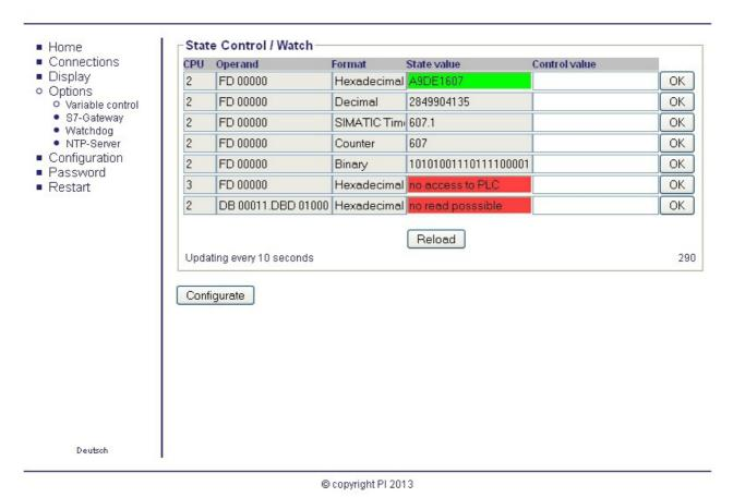
Controlling variables can always be opened with a configured password, and the configured status values can be read out. Do you want at a configured password transferred the control values in the PLC you are asked for the password. At incorrect or missing input the controlling of the variables is
