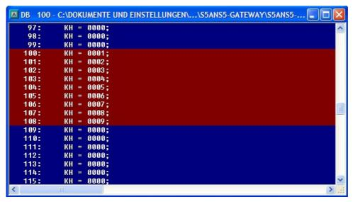
The marked bytes should be the same as the ones you have configured in DB10 of the S7 - PLC from DW0.
