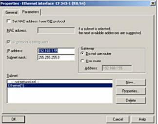
The subnet mask should fit to the given IP address (e.g. "255.255.255.0").
