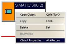
9. Type in the edit box "Name" the new name of the PLC (e.g. "S7-LAN-module/MPI-LAN-cable for CP mode"). Confirm the new name with a click on "OK".
