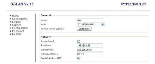
Agree the button "Send Gratuitous-ARP" and your device will send this ARP as the modul or the cable will recognize a link-state.
