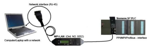
MPI-LAN connected with the computer using a switch or hub.
