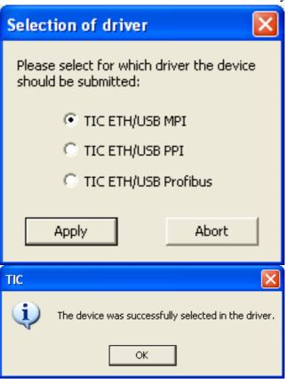
and confirm with "Apply". Now the driver for the module has been parameterized and the connection to the system can be established.
