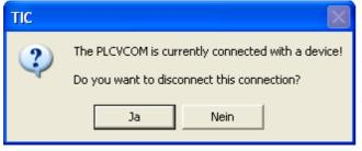
If the PLCVCom is connected to another module, this is indicated by a corresponding message. With "Yes" this connection is disconnected and rebuilt with the selected data.
