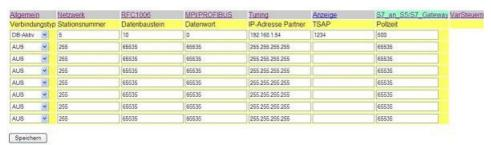
Lastly, you must now enter the number of your CPU that is stored in your PLC under "RFC1006" in "destination - CPU" and the "Bus" should be "Config".
