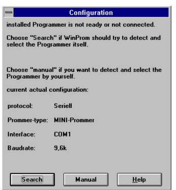
By pressing the operation button "search" the program tries to search and adjust the programmer automatically. First the programmers PG Prommer I, PG Prommer II, Multiprommer, FlashPrommer and Flash-Prommer II are searched on the serial interfaces. After that the MINI Prommer and then the Muliprommer are searched on the first parallel interface. If your programming device shoudn't be recognized, this is due to an inuse USB-Seriell Konverter. Therefor use the manual input!
