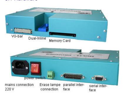
Connect the Multi-PROMMER with the provided serial or parallel cable to your PC. Connect the power cable to the Multi-PROMMER and then to a 230V socket. You can then switch on the MULTI PROMMER with the power switch.
