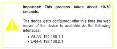
This message indicates that the device is currently not available under the current IP address (e. g. because the IP address, the WLAN network or the operating mode has changed). In the message you will see under which interface and IP address the device will be available in a few seconds. The web page will still try to reconnect to the web page periodically in the background.
