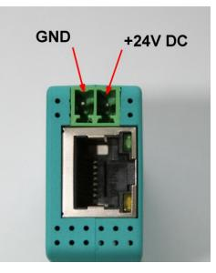
Before using the external power supply, check the correct pinning of the Phoenix plug! The module itself is protected against wrong pinning the phoenix plug, but we can not guarantee for protection for the possible connected assemblies.
