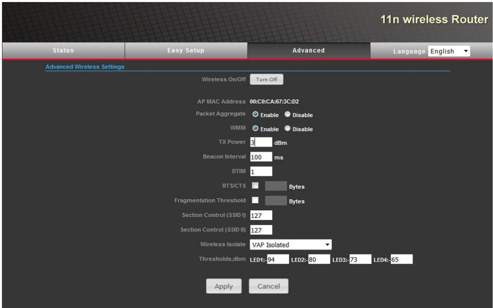
Within the "Wireless On / Off" option you can use the "Turn On / Off" button to turn on/off your wireless network. Below it shows the MAC address of the access point. Furthermore, it is possible to turn on/off the " Packet Aggregate " and the "WMM".
