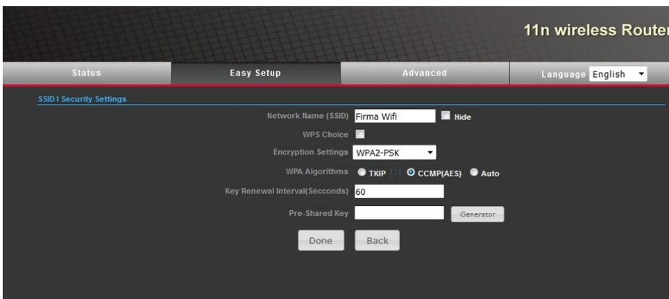
The screenshot shows the '11n wireless Router' configuration interface, specifically the 'SSID Security Settings' section. The 'Network Name (SSID)' is 'Firma Wifi' with a 'Hide' checkbox. The 'WPS Choice' checkbox is unchecked. 'Encryption Settings' is set to 'WPA2-PSK'. Under 'WPA Algorithms', 'TKIP' is selected. 'Key Renewal Interval(Seconds)' is set to '60'. There is a 'Pre-Shared Key' field and a 'Generator' button. At the bottom, there are 'Done' and 'Back' buttons.
