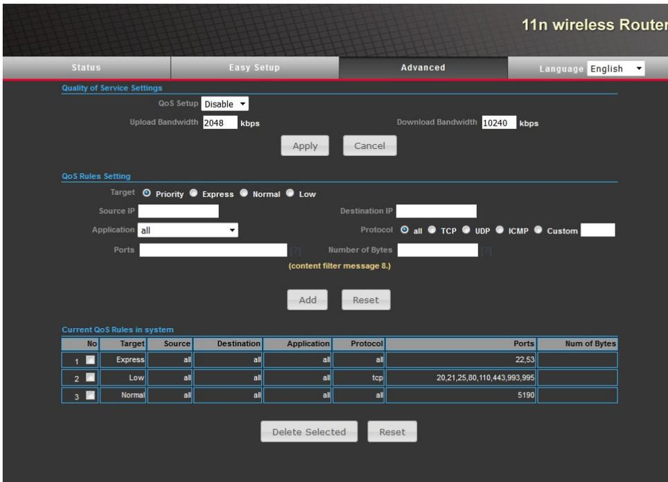
To use QoS, you must set the QoS settings to "Enable", specify the bandwidth of Download and Upload and accept by clicking "Apply".
