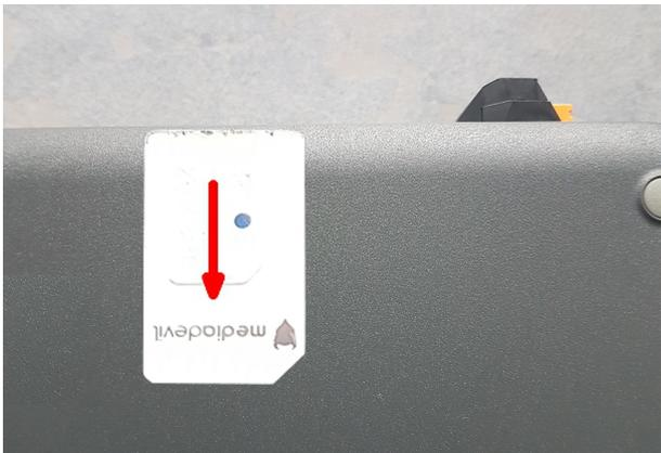
Insert the SIM card with the contact side facing down (slanted corner at the front right) into the slot until it clicks. Pressing again releases the card and it can be pulled out.
