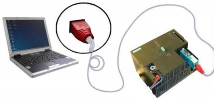
Before you can use the device you have to connect it properly. In the first step you should put your device on the MPI/Profibus interface of your PLC. If a bus cable is already connected to the interface of your PLC you can simply connect your device on top of the cable if a diagnostic jack is available. Alternatively you can also put your device on a slave module (e. g. a panel).
