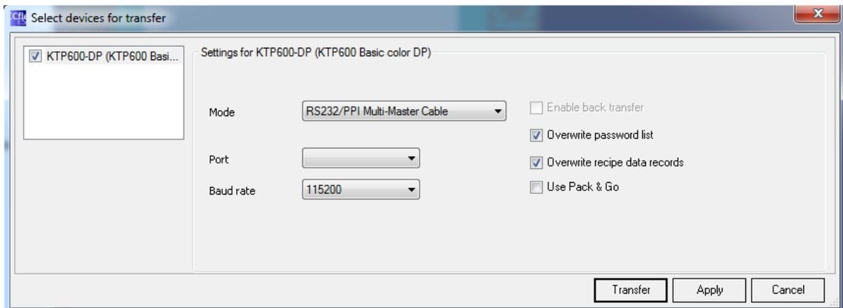
There you then have to make sure that your operating terminal is checked and selected on the left side. Afterwards you have to set up the mode “MPI/DP” on the right side as well as the station address from the operating terminal.
