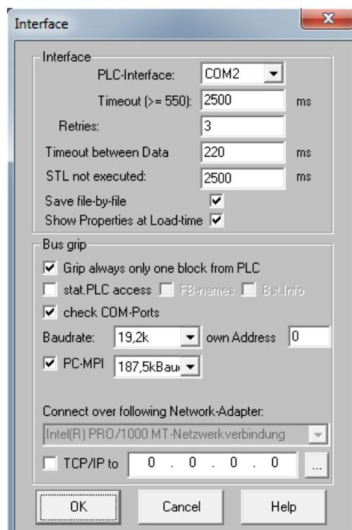
On the selection “PLC-Interface” on the top of the window you can then select your COM port which should be used for the communication. This COM port can either be a physical COM port for the communication with a MPI-II cable or a virtual COM port from the PLC-VCOM application for the communication with any of the USB or LAN devices. When you want to communicate with a LAN device you can also do this without any further driver or software. Therefore you have to enable the option
