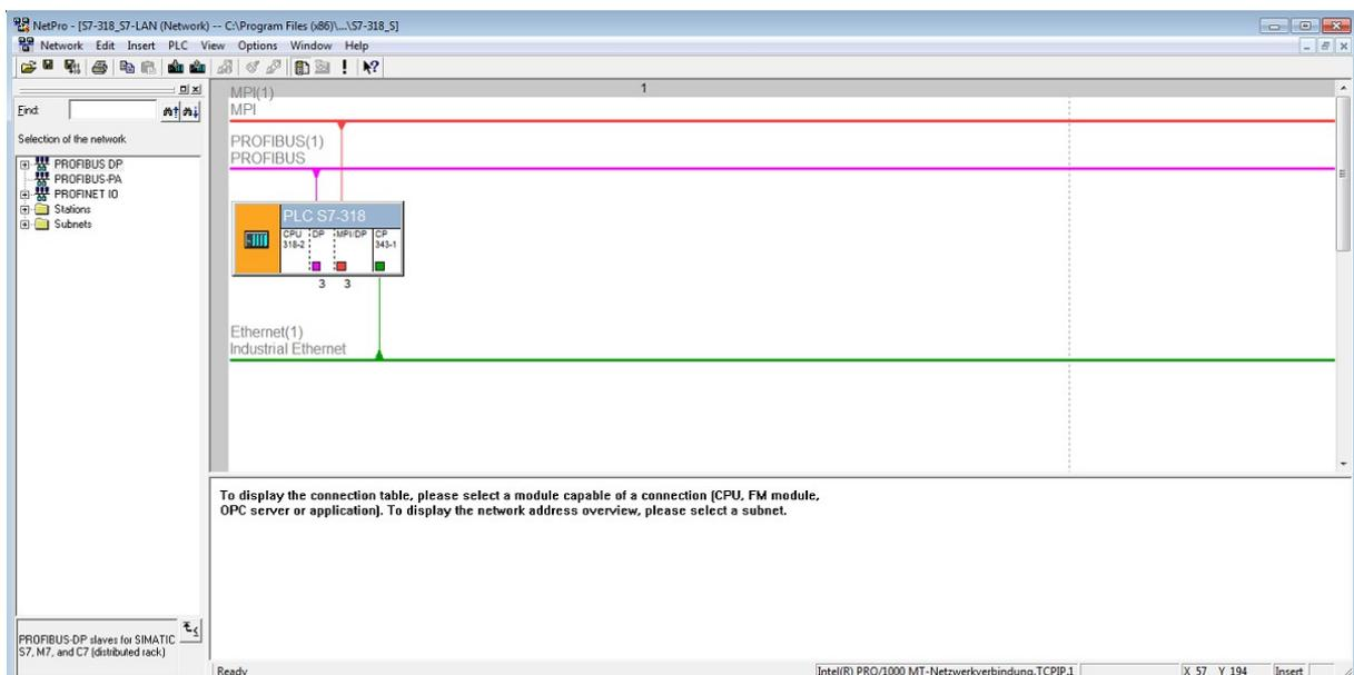
In the next step you should save and compile your configuration again. Thereby the program also checks for possible errors or problems. When no errors occurred you can then download the configuration as well as your S7 program (only if needed) into your PLC.
