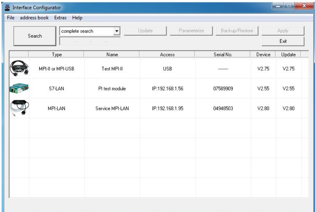
By default the TIC searches for all devices, which are connected to your PC or network, when starting the program. By clicking on the button “Search” a new search can be executed at any time. If you want to search only for a specific device type or via a specific interface, you can
