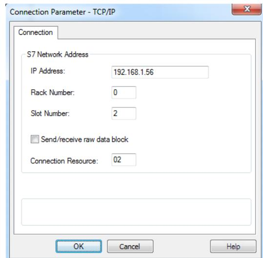
When this data is configured too, you can close the dialog by a click on the button “OK”. In the next step you can then create and configure variables within the list view.
