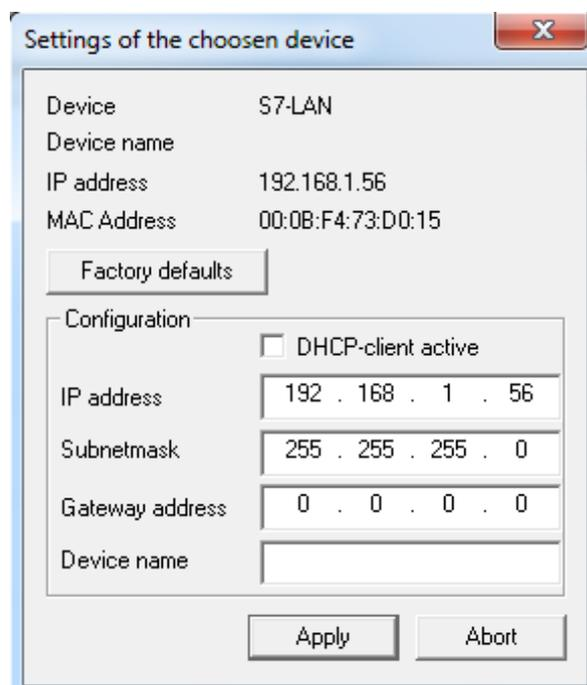
On this dialog you can configure another fixed IP address for the device or enable the DHCP option (this needs a DHCP server on your network) as well as setting a name for the device. The name of the device is used for easier identification only.
