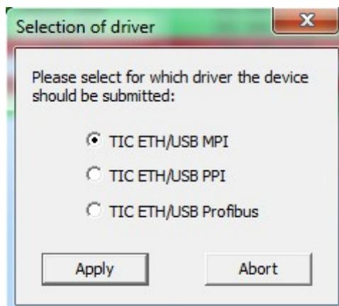
When you have selected a S5-LAN module, the module can be set up for the usage together with the PLC-VCOM. After you have clicked on the button “setup communication”, the program will check if the PLC-VCOM is installed on your PC and not too old. After that the TIC will start the PLC-VCOM (if not already started) and then lets the PLC-VCOM connect to the specified device. Next the TIC waits for the response and finally shows you a message with the current state:
