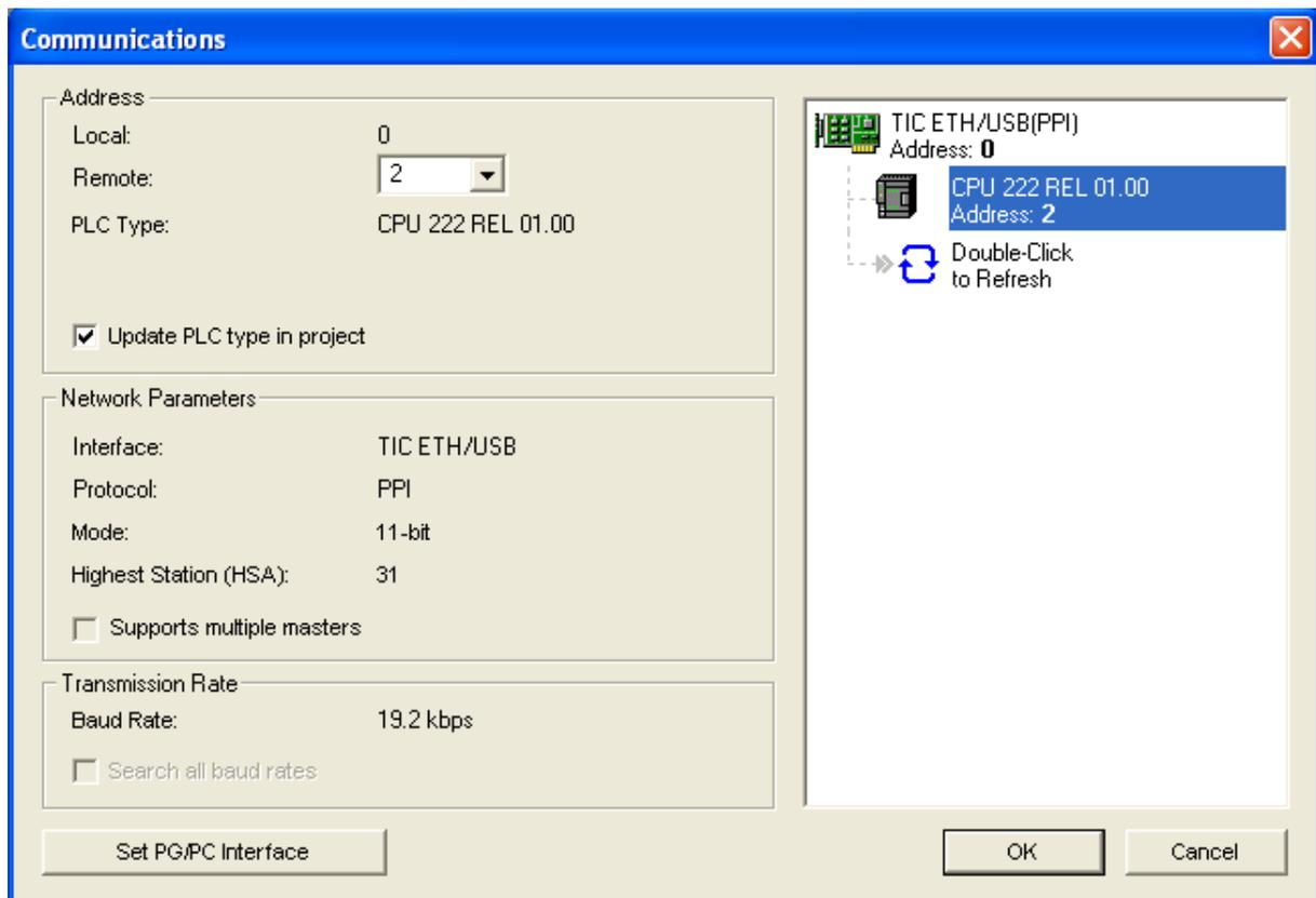
To submit the PLC for the communication you will have to select it on the right side and then click on the button “OK”. Afterwards you can use your MicroWin application normally for the communication with your PLC (e. g. loading a program or viewing and controlling variables).
