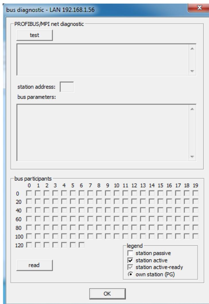
When you click on the button “test” a connection to the device and bus will be tried to establish. If an error occurs thereby this will be shown on the first field. Otherwise the collected information about the bus (baud rate, profile, bus times, etc.) as well as the own station address will be shown.
