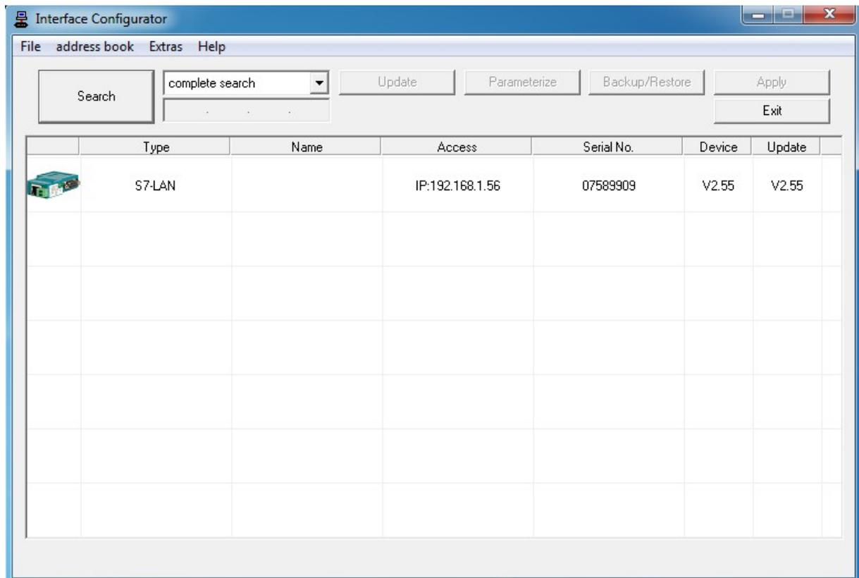
When your device was found you can execute a double click on the cell with the IP address of the corresponding device entry. Now a dialog with the network settings of the device should appear:
