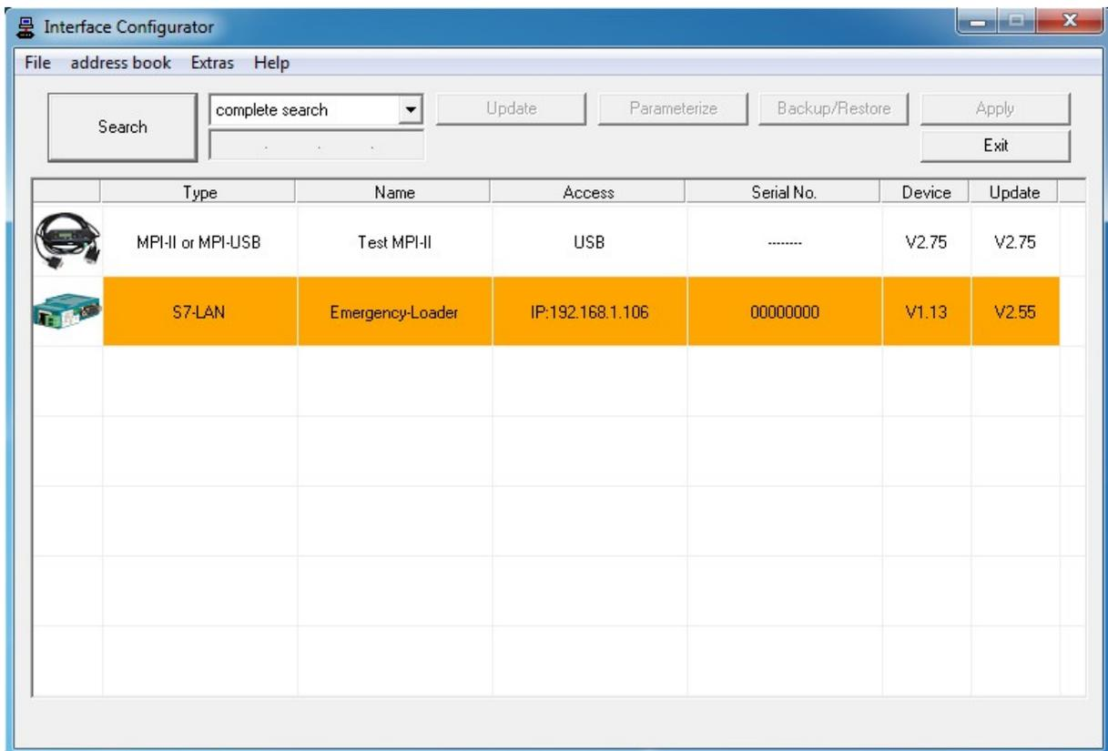
Devices who are in the emergency loader are colored in orange and assign them the next free IP address from the PC to itself automatically (only for LAN devices). The update can be executed normally by first choosing the device and then clicking on the button “Update”.
