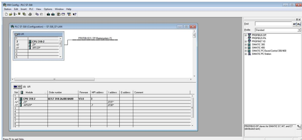
In the next step you can then add a CP (e. g. SIMATIC 300 → CP-300 → Industrial Ethernet → CP 343-1 → 6KG7 343-1EX10-0XE0 → V1.0) from the hardware catalog to your station. Afterwards the dialog with the properties of the CP will be opened automatically. On this dialog you have to enter the IP address and the subnet mask from your device. Furthermore you can also create a new Ethernet subnet or assign the the CP to an already existing subnet.
