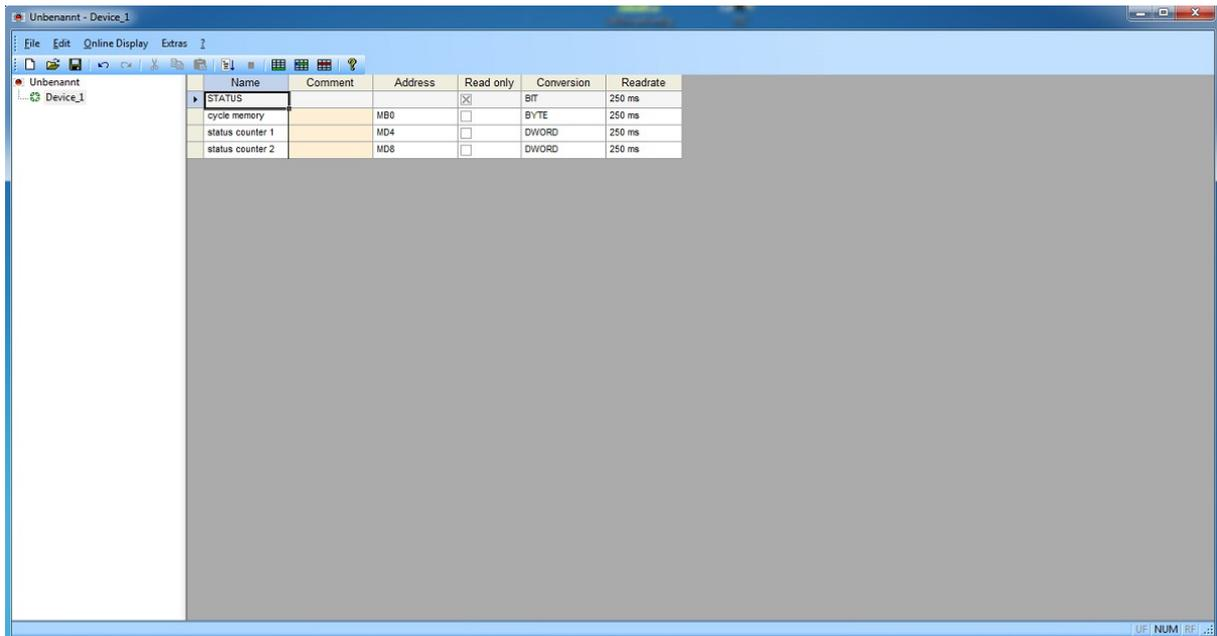
With a click on the menu entry “Online Display” → “Start Online Display” you can then finally switch to the online view. Thereby the configured items gets retrieved from the device within the configured cycle and shown on the main window:
