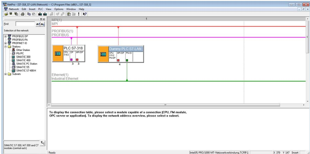
In one of the last steps you should save and compile the configuration again. If an error while compiling occur you should check all done settings again. Otherwise the configuration can be downloaded to the real existing controller. The transmission of the configuration to the Dummy PLC isn't possible and also don't needed.
