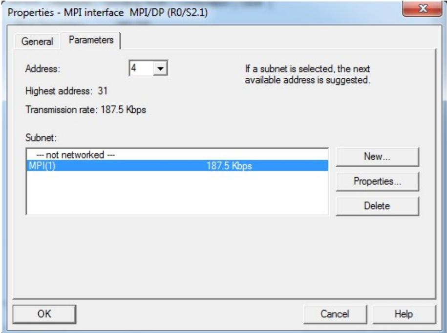
Now you can close both property windows, save the configuration and close the hardware configuration program. Afterwards you should see the NetPro window again. There you should then see your configuration of the Dummy PLC as well as the connection on the MPI/Profibus:
