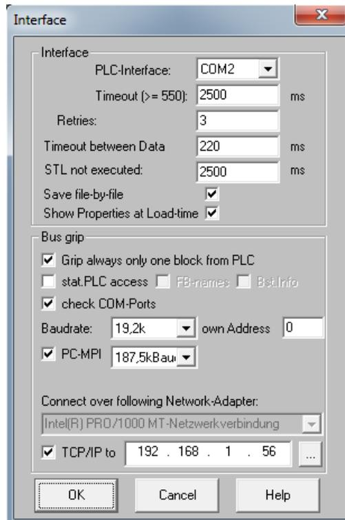
If all settings are set up you can submit the parameters with a click on the “OK” button. Now you can click on the menu entry “File” → “Open” → “PLC” to read in the list of blocks within your PLC. In some cases a small window will appear where you have to select to which destination CPU you want to connect to:
