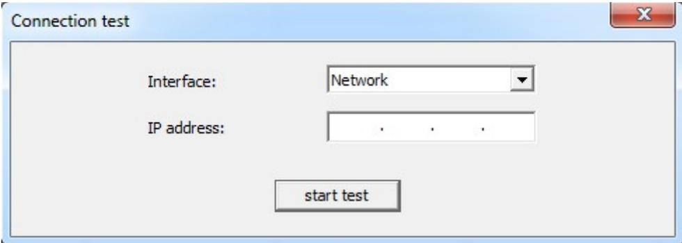
After you have selected the interface and entered the IP address you can click on the button “start test”. Depending on the connection the test may be finished in a few seconds. The process as well as the result will be shown within the window.
