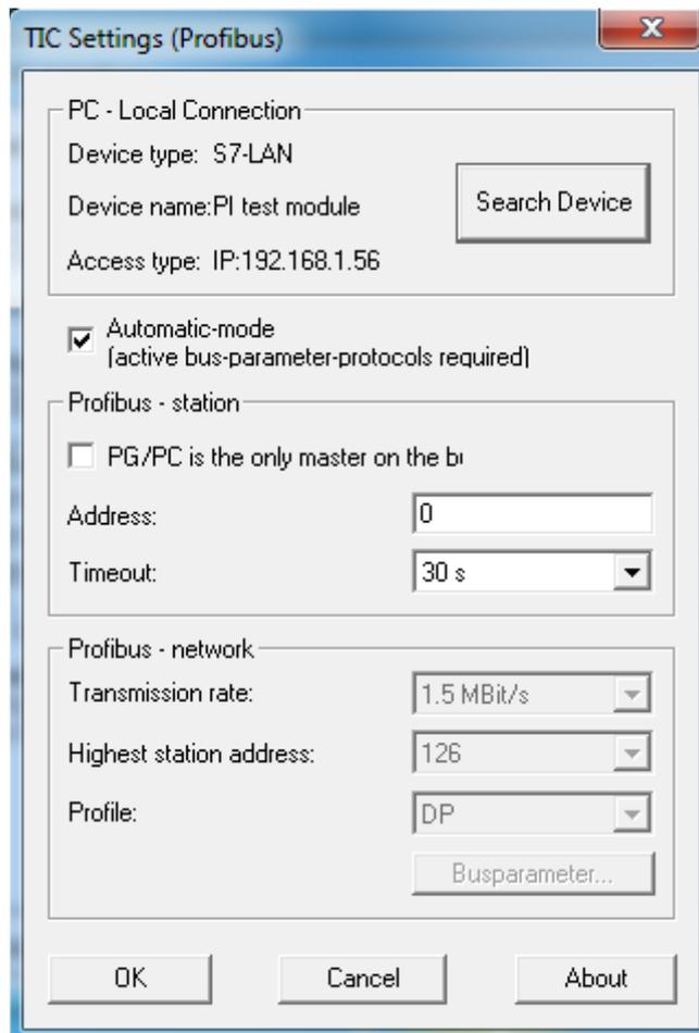
Within the section “Local Connection” you can see which device is currently selected for the communication with this interface. If you want to use another device you have to click on the button “Search Device”. Thereby the interface configuration tool of the TIC gets opened where you can search for devices and then select the device you want to use. Finally you have to click on the “Apply” button. Afterwards you will be redirected back to this properties dialog.
