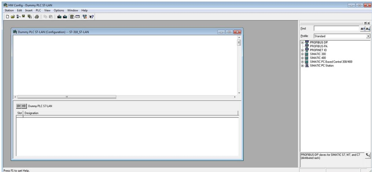
For adding new modules into the hardware configuration you have to add a rail (SIMATIC 300 → RACK-300 → Rail) from the catalog first. Afterwards you can add a PLC with integrated network connection (e. g. SIMATIC 300 → CPU-300 → CPU 315-2 PN/DP → 6ES7 315-2EG10-0AB0 → V2.3). Subsequently you should get a dialog with the network properties of the PLC. There you then have to enter the IP address and subnet mask from your LAN device:
