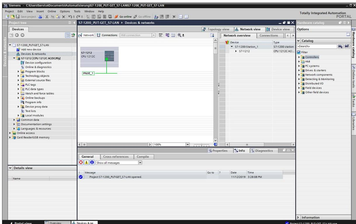
In the next step you should click on “Connections” within the control line above the device view. Furthermore you have to select “S7 connection” on the field on the right side. Then you can execute a right click on your
