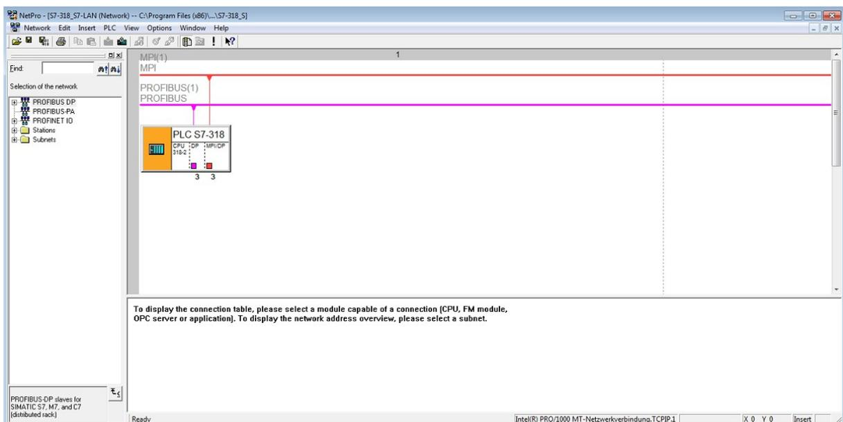
Afterwards you have to execute a double click on the SIMATIC 300/400 Station where the LAN device is connected to. Thereby the hardware configuration gets opened. This should then look similar to the following:
