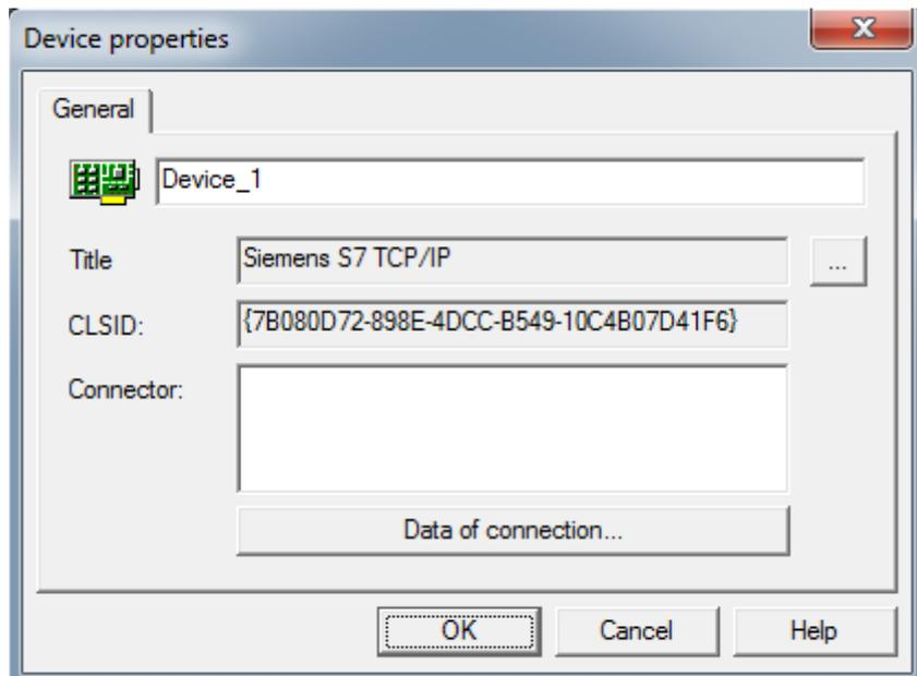
To specify further settings for the connection you have to click on the button “Data of connection”. There you then can configure the IP address or COM port as well as some more settings depending on the used access type.
