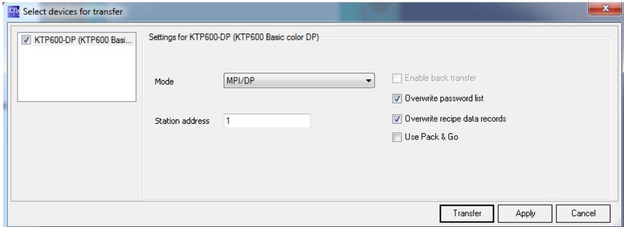
If all settings are correct you can click on the button “Transfer” to transfer the project into the operating terminal. The button “Apply” can be used to save the settings without executing a transfer to the terminal. This for example may be needed if you want to update the operating system from your operating terminal without transferring your project first.
