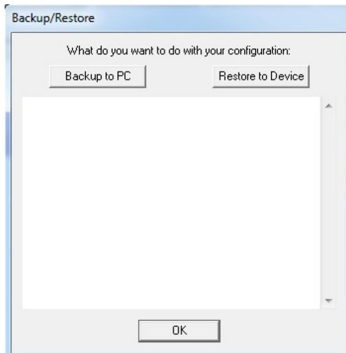
When you want to create a backup of the configuration you have to click on the button “Backup to PC”. Now the configuration from the device gets retrieved. After that you have to select a folder and enter a file name where the configuration should be stored.
