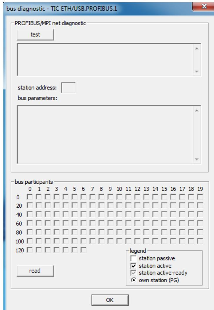
In the first step you should make sure that the connection to the device and bus is working correctly. Therefore you have to click on the button “Test”. After a few seconds the state will be displayed on the first text area. If the connection was successful the station address as well as the bus parameters will be shown within the two text fields below too.
