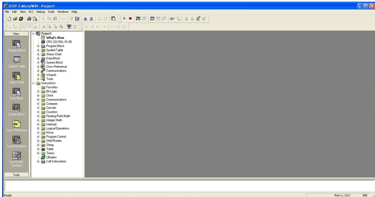
If the interface is configured you will have to set up the communication to the controller. Therefore you have to click on “Communications”. This item can also be found within the block “View” on the navigation bar on the left side of the program. After you have clicked on the item you should get the following dialog:
