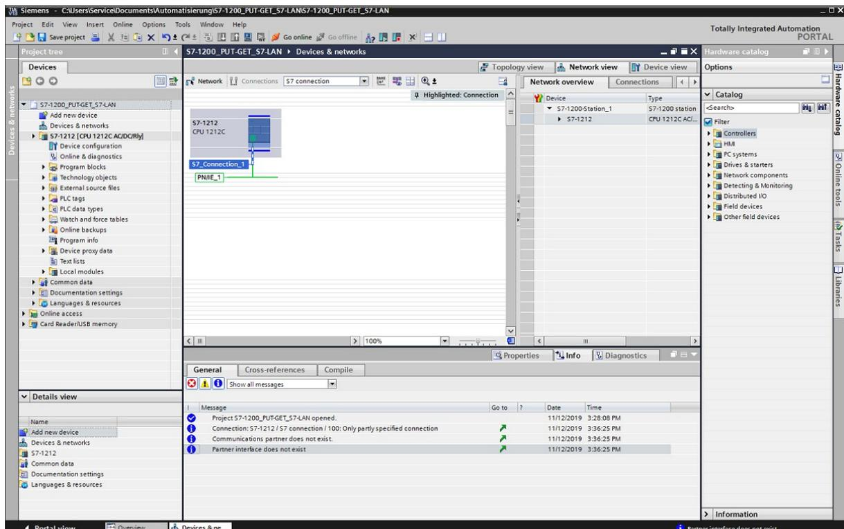
Now you can open the properties area and navigate to the tab “General” and then to the category “General”. There you have to configure the IP address of the partner device. When needed you can also assign a name to the connection and device.
