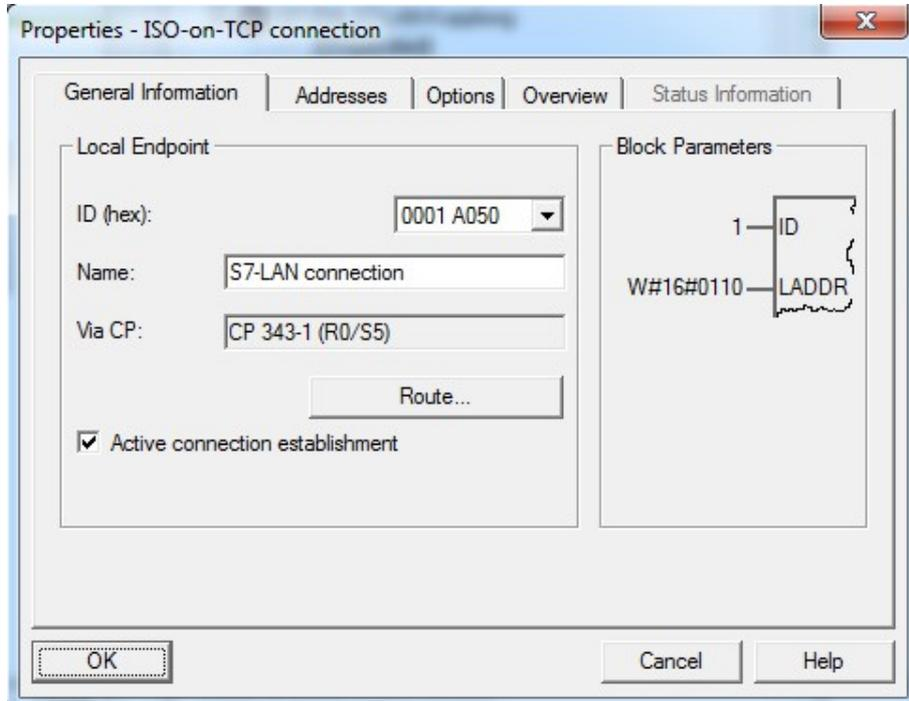
In the next step you should navigate to the tab “Addresses”. There you have to configure the IP address of your LAN device as the Remote IP as well as both TSAP values. But keep in mind that the TSAP values have to be crossed with the configuration on the S7-LAN. This means the “Local TSAP” within the S7-CP equals the “Dst. TSAP” within the LAN device and the “Partner TSAP” equals the “Src. TSAP”.
