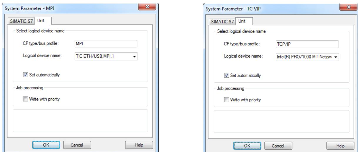
When these settings are checked and the dialog is closed again you can add a new connection. Therefore you have to execute a right click on the corresponding entry within the protocol suite again and then choose “New connection”. After that an entry on the navigation bar on the left side is created automatically and you will have to enter a name for that connection.
