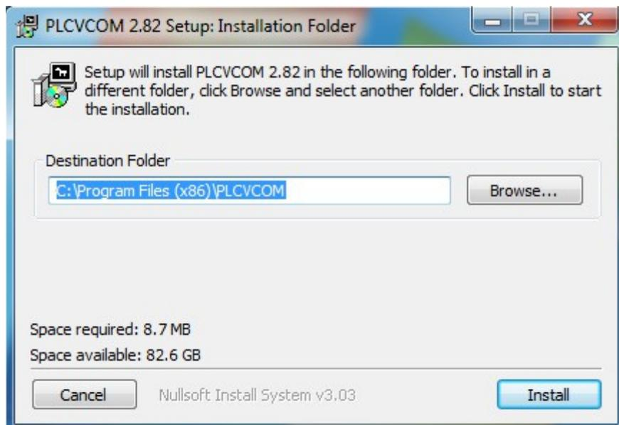
After you have clicked on “Install“ the process of the installation will be started. Before and while the installation is running some examinations are done by the installer. The setup assistant will guide you through the whole process of the installation and tells you, if you should take action.
