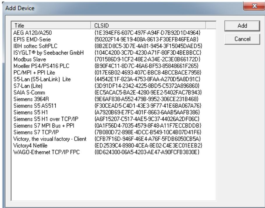
In this dialog you then have to select “Siemens S7 TCP/IP” when you want to access your LAN device directly via network or “Siemens S7 MPI Bus + PPI” when using serial access (with the MPI-II or a virtual COM port from the PLC-VCOM application). Then you can click on the “OK” button. Afterwards the dialog with the device properties gets shown:
