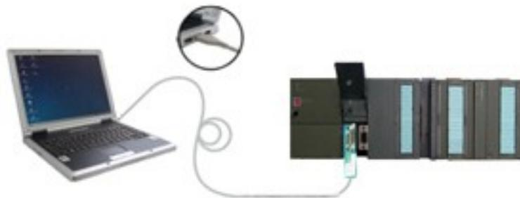
In the first step you should put your USB device on the PPI/MPI/Profibus interface of your PLC. If a bus cable is already connected to the interface of your PLC you can simply connect your device on top of the cable if a diagnostic jack is available. You can also put your device directly on a slave module (e. g. a panel) if you don't want to work on a bus with a controller.
