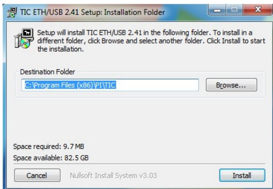
When you have clicked on the “Install” button, the installation process gets started. Before and while the installation is running, some tests are getting executed (e. g. for an older version). The installation assistant will guide you through the whole process and shows you the current state.
