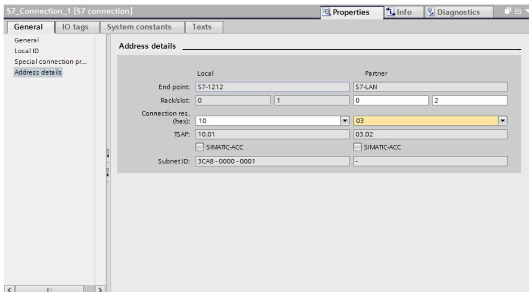
On the next step you have to expand your PLC program by calls to the PUT/GET functions. The correct connection number can be found within the properties of the connection. If this connection is the first one, the ID as a general rule should be 16#100.
