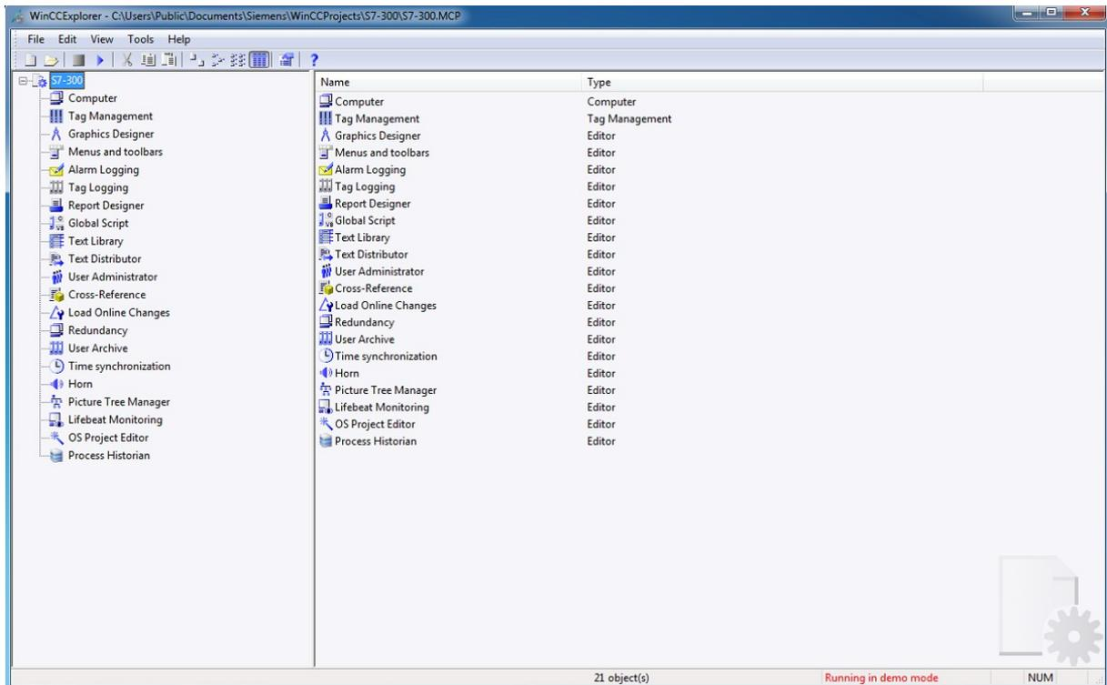
When WinCC is opened you can execute a double click on the entry “Tag management” within the navigation bar to open the management tool for tags. There you then have to add the protocol suite for SIMATIC S7 first if not done already. The suite can be added with a right click on “Tag Management” and then navigating to “Add new driver” → “SIMATIC S7 Protocol Suite”.
