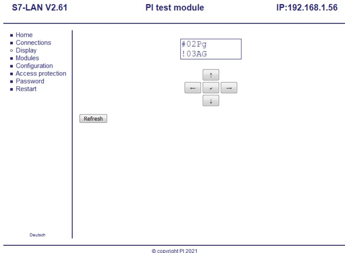
The display can be controlled with the five buttons below the viewed display. An explanation about the content of the display as well as of the operation can be found within the section “Keyboard and LCD display” in this chapter.
