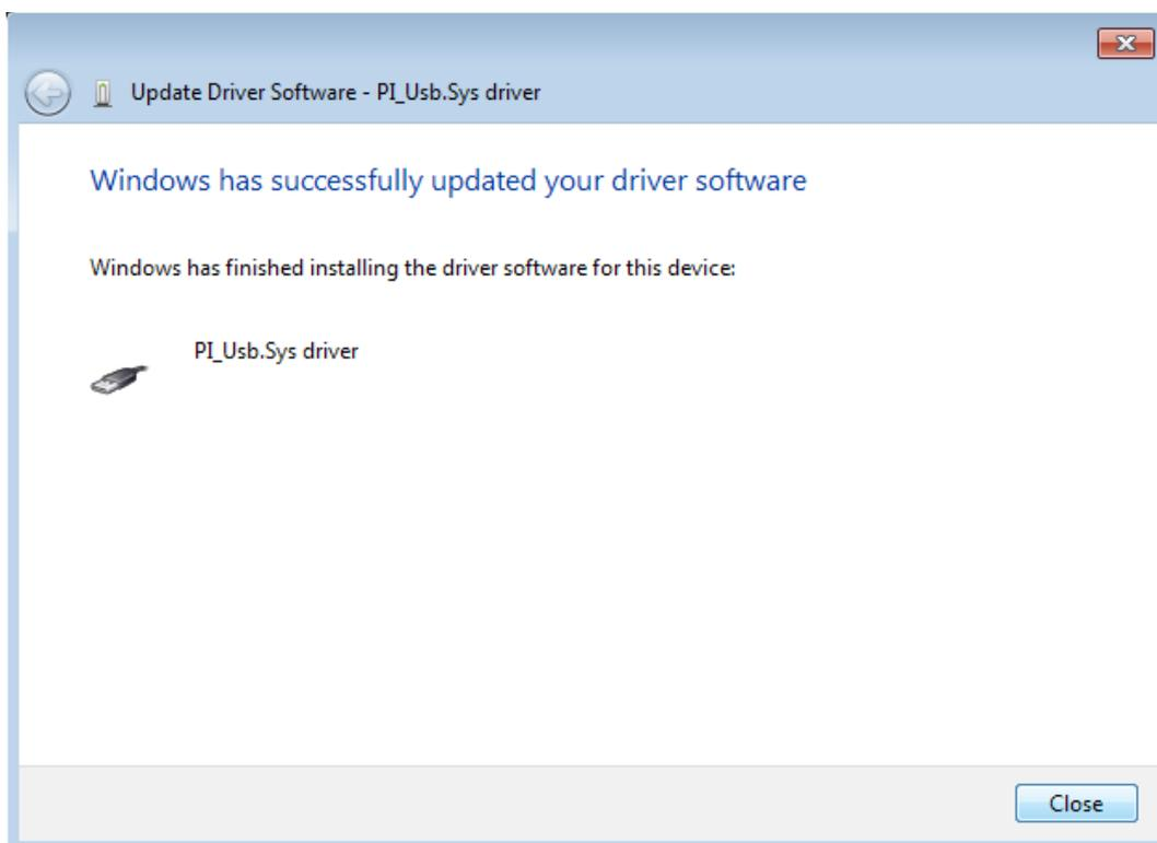
Now you can go back to the main window of the Device Manager and check if the entry “PI\_Usb.Sys driver” within the section “Universal Serial Bus controllers” was created. This entry shouldn't have an exclamation mark anymore.
