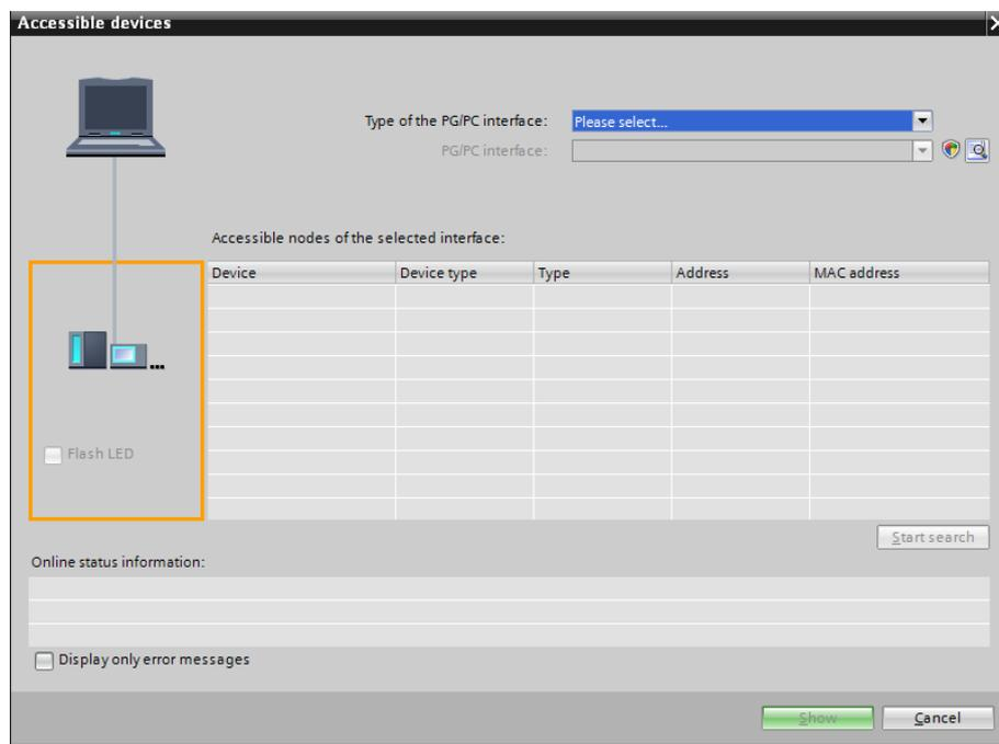
Within this dialog you then have to choose the type of the PG/PC Interface as well as the driver or interface which should be used. The selection here is a bit different from the classical PG/PC Interface dialog. When you have finished your selection you can click on the button “Start
