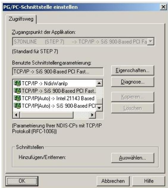
3. Select under "used Interface parameterization" the entry "TCP / IP => XXX", where "XXX" for the used network card.
