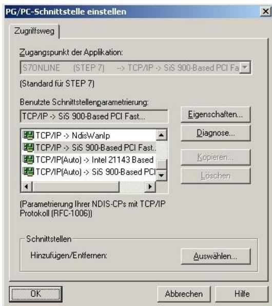
3. Select under "Used Interface". The entry "TCP / IP => XXX", where "XXX" is for the used network card.
