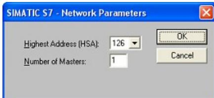
6. The button „More ...“ leads you to a small dialog where the „Highest Station Address“ should be configured to „126“. Set up the „Number of masters“ (e.g. „1“)
