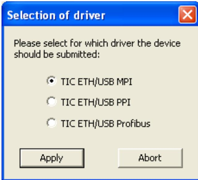
and confirm with "Apply". Now the driver for the module has been parameterized and the connection to the system can be established.
