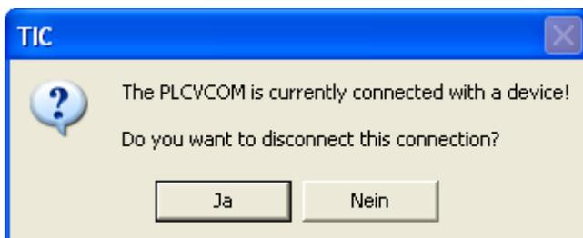
If the PLCVCom is connected to another module, this is indicated by a corresponding message. With "Yes" this connection is disconnected and rebuilt with the selected data.
