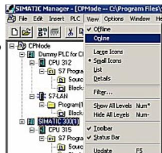
36. To test the communication open the branch of your real existing PLC (e.g. “SIMATIC 300(1)”). The branch below the PLC is the CPU Type (e.g. “CPU 315“). A additional red symbol is displayed next to the standard CPU symbol. Open this branch, too. The next branch you should open is named as „S7 Program“ (e.g. “S7 Program(3)”). Finally click on “Blocks” to get a complete list of available blocks from your PLC.
