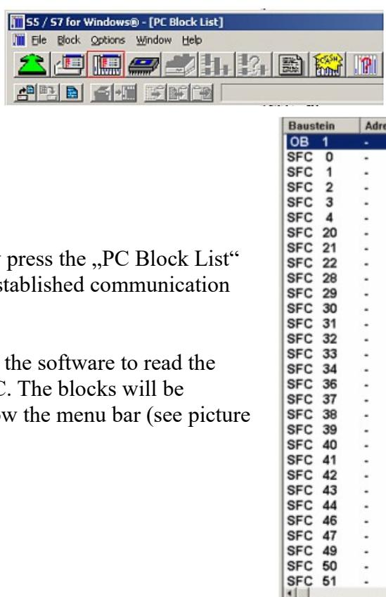
7. Back in the main window press the „PC Block List“ button for testing the new established communication configuration.
