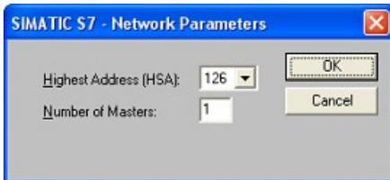
6. The button „More ...“ leads you to a small dialog where the „Highest Station Address“ should be configured to „126“. Set up the „Number of masters“ (e.g. „1“)
