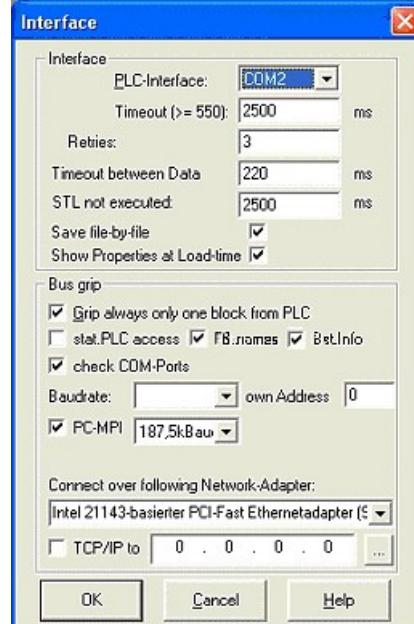
3. A dialog appears, in which you are able to set the “AG-Interface” (COM-port) in the section “Interfaces”.
