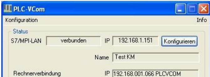
5. After a successful connection, in the main window of the PLC VCOMs appears the cable type with which the computer connects, the connection status is "connected", the IP address and the name of the connected participant and the existing connections to the cable / module.
