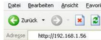
1. Start the Web – Browser and enter in the address line “http://” and the IP address from the module you are using. The IP address is shown in the PLC-VCOM software. Confirm with ENTER to load the main page (Select language).
