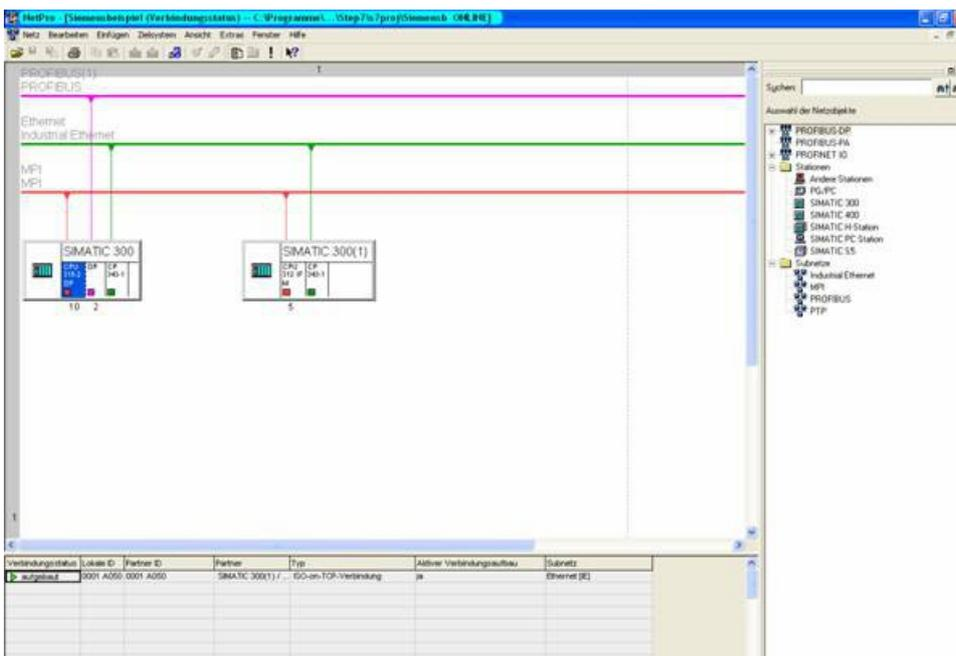
9. Now you have to adjust the "Configure Hardware" as with the S7 PLC before. There you add the same CP as in the first and of course the CPU of the PLC. The CPU and the CP (see 5 - 7) you adjust in the same manner as before. Download the configured stations in the respective PLCs after configuration.
