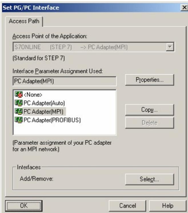
4. Press "Select" to add the RFC1006 required elements to the PG / PC - interface configuration.
