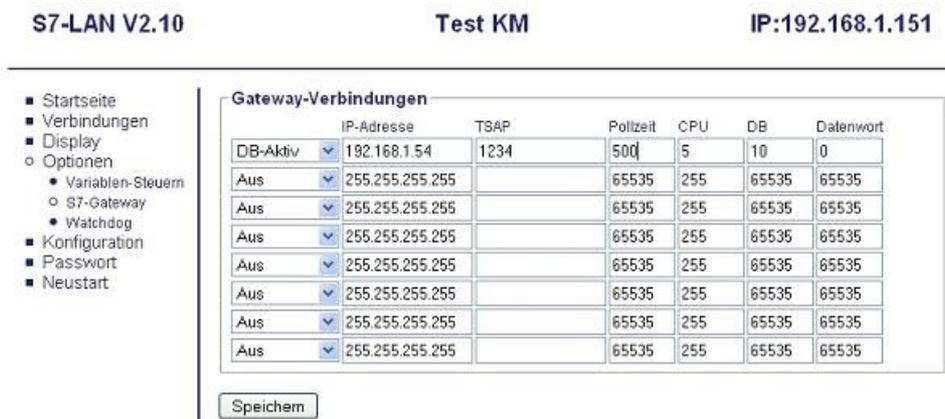
The last step is to configure the gateway. Here you have to adjust at "Connection Type", "DB - Active" (the partner device "passive") and at "Station Number" you have to deposit the number of your PLC. Now you should decide which is the configuration data block in your PLC and from which data word. The IP - address of your S5 - LAN you enter in the field "IP - address partner". In "TSAP" you deposit only the same name as you have assigned in S5 - LAN Manager to your S5 - LAN.
