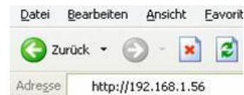
If you don't know the IP-Address of your S7/MPI-LAN, you can open the PLC software to find out the address. At configuration, you can display all connected devices (on PC or network). More about that on section „PLC - VCOM“.
