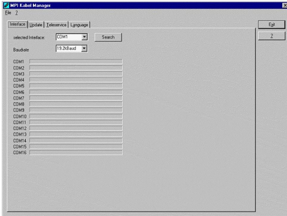
In „set interface“ you can choose the COM-port your device is connected at. Only the COM-port which was active at starting the MPI-Kabel-Manager are shown.
