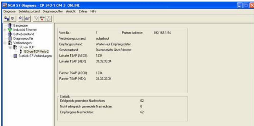
4. For added control, you can now take the DB10 in your S7 - SPS (with CP) and take the DB14 in your S7 - SPS (with S7 - LAN gateway), and check if the values of the 20 bytes you have configured in the each other PLC in DB10 and DB14 from DW0, match with those from DW100. If that is the case, the communication between S7 and S7-CP-LAN was completed successfully.
