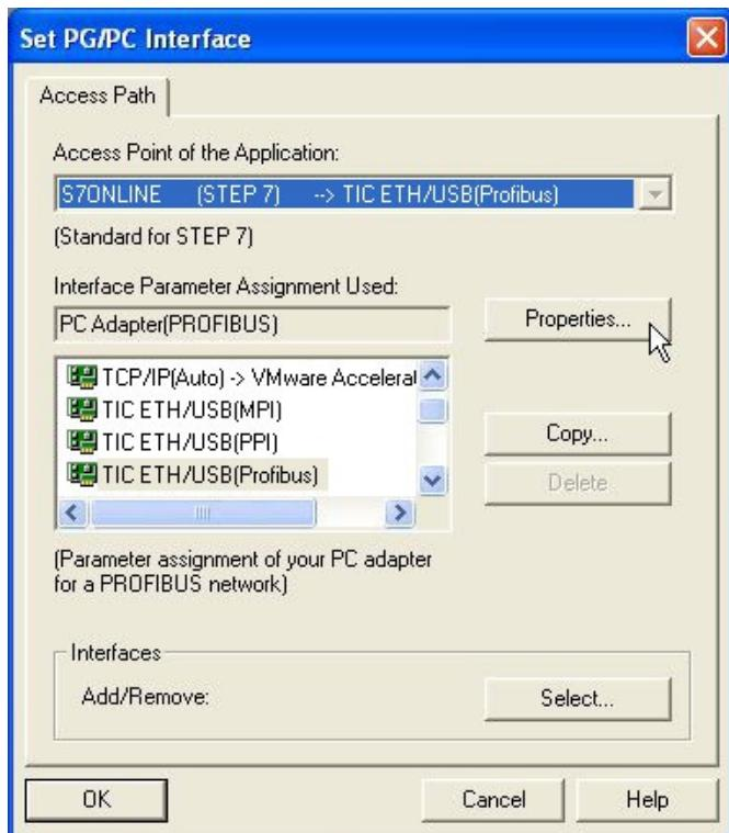
18. If you want to use ProTool/Pro RunTime you can set the "PG/PC Interface" by selecting the entry "DPS7ONLINE". Therefore you have to select "Access Point of Application" and configure it as described above. The easiest way is to use the S7-LAN/MPI-LAN/MPI-USB- driver which supports USB and LAN products.
