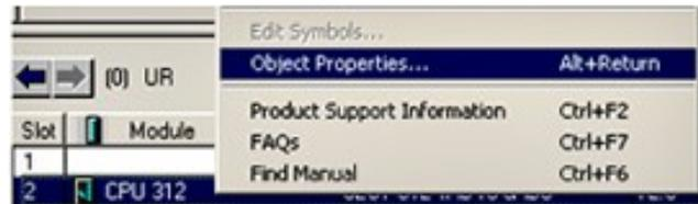
27. In the dialog “Properties – CPU 312 - (R0/S2)“ press the “Properties...” button. In the new dialog you can assign the MPI address to the CPU and choose the subnet the CPU should use.
