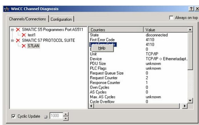
20. The tool could not detect a running connection so it marked the connection/s with a red 'X' (registry card "Channels/Connections").
