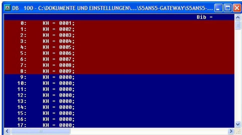
2. Save the blocks and set the inputs E8.0 and E9.0 to "1" in your PLC with the active S5 - Gateway module and restart the cycle.
