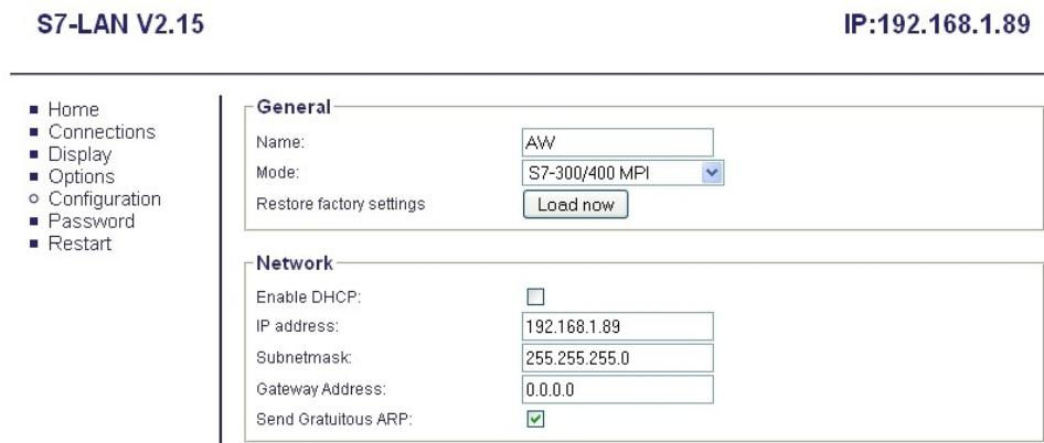
Agree the button "Send Gratuitous-ARP" and your device will send this ARP as the modul or the cable will recognize a link-state.
