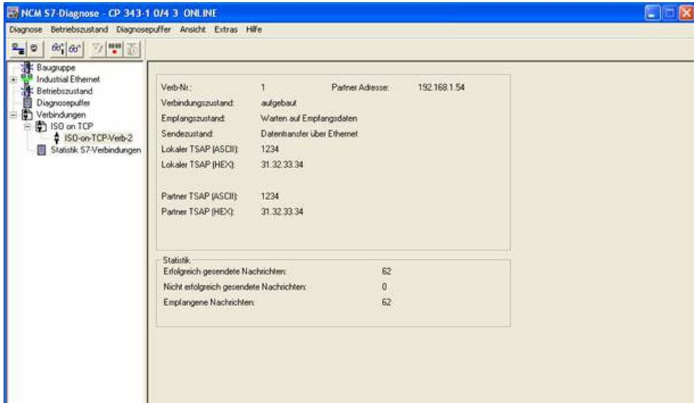
6. Now open the DB100 in your S5 - PLC and the DB10 in your S7 - PLC and check if the values are consistent with those from DW100 of the 20 bytes that you configured in the other PLC in DB100 and DB10 from DW0. If that is the case, the communication between S5 and S7 was successfully completed.
