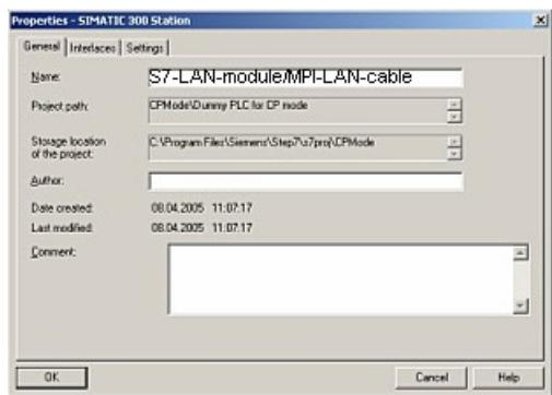
9. Type in the edit box “Name“ the new name of the PLC (e.g. “S7-LAN-module/MPI-LAN-cable for CP mode“). Confirm the new name with a click on “OK“. The rectangle should be updated by the application.
