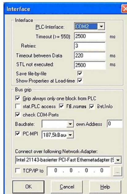
4. Configure the baud rate in the section "Bus access" to "19,2k". Below change the value for PC - MPI to "187,5kBaude".
