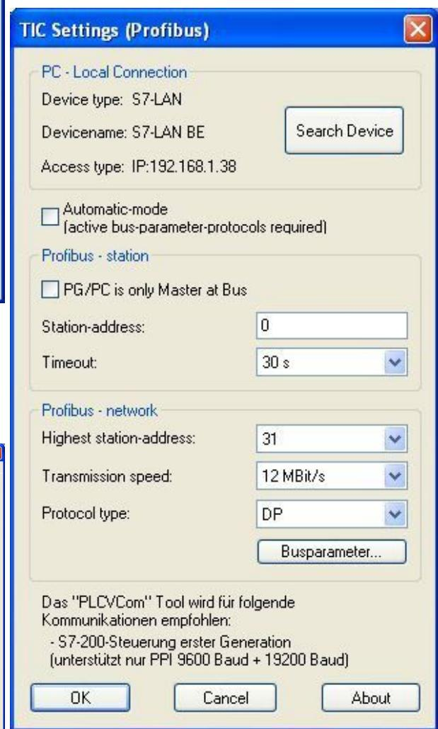
9. Is the device-type is not identical with your used device, search for your device with "Search Device". Select the device in the result windows and click on the button "Apply".
