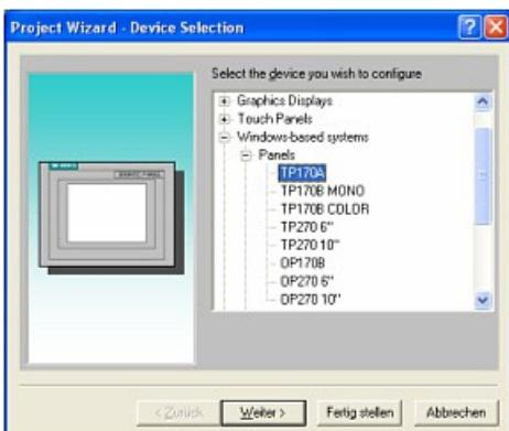
4. „Next“ leads you to a new dialog. Type in the specific fields the name of the PLC device and choose the used PLC in the driver selection (e.g. „SIMATIC S7 – 300/400 V6.0“).
