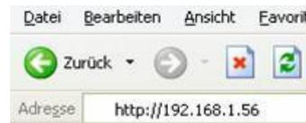
Start your Web browser and enter the IP address of the module in the address bar with the preceding "http://". Confirm with the <ENTER> key to load the Main page (Language selection).
