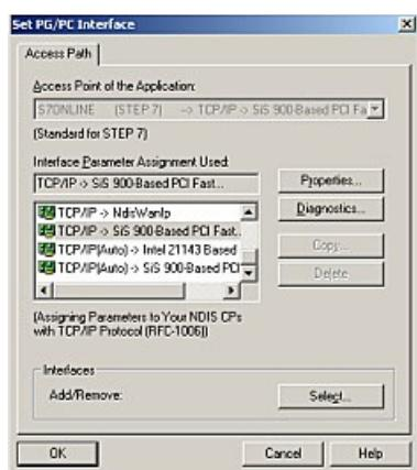
For the Step 7 software version 5.2 you need the SIMATIC NET package, otherwise the Step 7 software will not show the desired entries (TCP/IP, etc.) because it is not supported.
