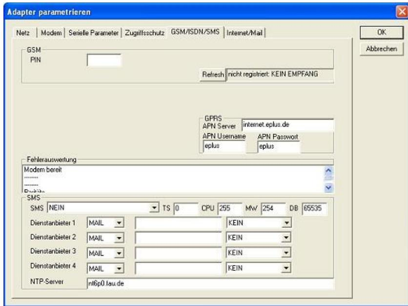
**PIN:** PIN-Number of the SIM-Card, up to 8 numeric chars, (only for TELE-SERVICE GSM).
