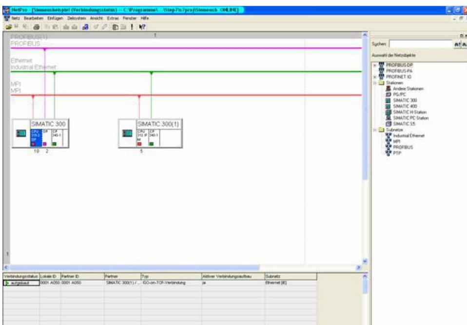
9. Now you have to adjust the "Configure Hardware" as with the S7 PLC before. There you add the same CP as in the first and of course the CPU of the PLC. The CPU and the CP (see 5 - 7) you adjust in the same manner as before. Download the configured stations in the respective PLCs after configuration.
