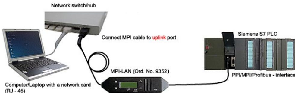
**MPI-LAN Connection possibilities with operator panel**
