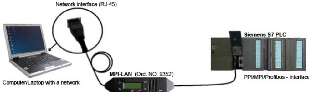
**MPI-LAN connected with the computer using a switch or hub.**
