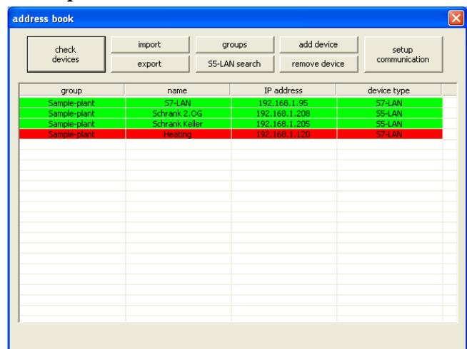
The entries in the address-book marked in green color are immediately accessible. If a module has a red background, then no communication can be established. This can happen, for example, through a non-active VPN-connection. In this case, set up the VPN-channel and check the accessibility of the
