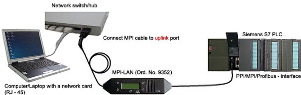
MPI-LAN Connection possibilities with operator panel
