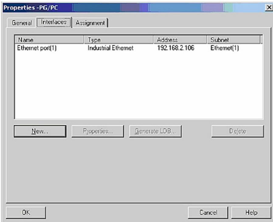
16. Select the registry card “Assignment“ and mark “Ethernet port(1)” by using the list “Configured Interfaces:”. In the list “Interface Parameter Assignments in the PG/PC:“ choose “TCP/IP - > XXX“. “XXX“ stands for the network interface card you want to use.
