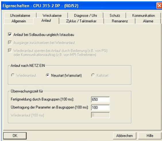
10. In your network configuration you can open the object configuration of your cpu. Here you can find the option "shall escape" and "equal to actual configuration". The mark on checkbox should be set.
