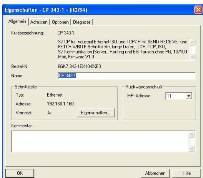
9. Now your CP is integrated on the CPU. With doubleclick on CP you can see the objectconfiguration. Here you have to configurate the rear panel connectors. The address should be 1 higher then the MPI/Profibus address of your S7/MPI-LAN
