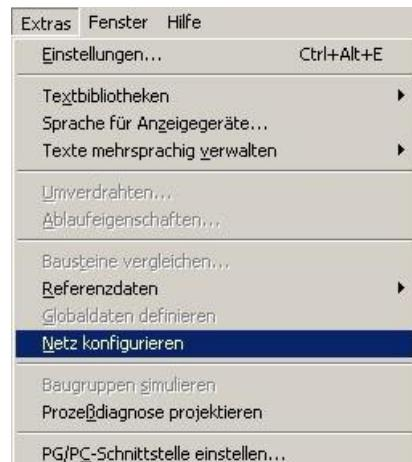
4. Back to the main window of Step7 software you can configurate your network at menu „Extras“, „Configure Network“.
