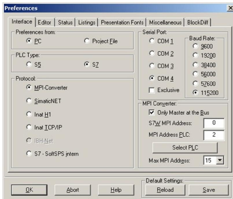
3. Choose the first registry card „Interface“ (standard) and set up the configuration data as described below:
