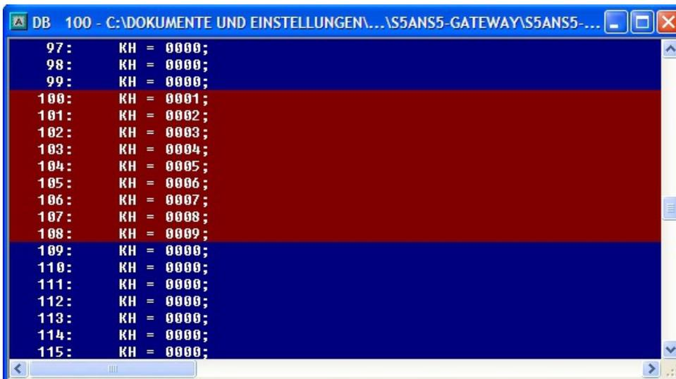
The marked bytes should be the same as the ones you have configured in DB10 of the S7 - PLC from DW0.
