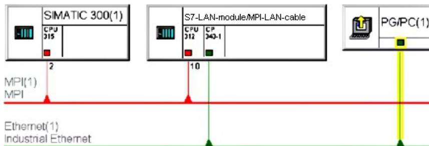
32. The last thing you have to do before the connection is established is to configure the S7-LAN module.
