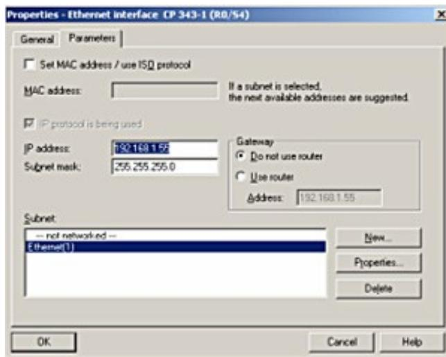
The subnet mask should fit to the given IP address (e.g. “255.255.252.0“).
