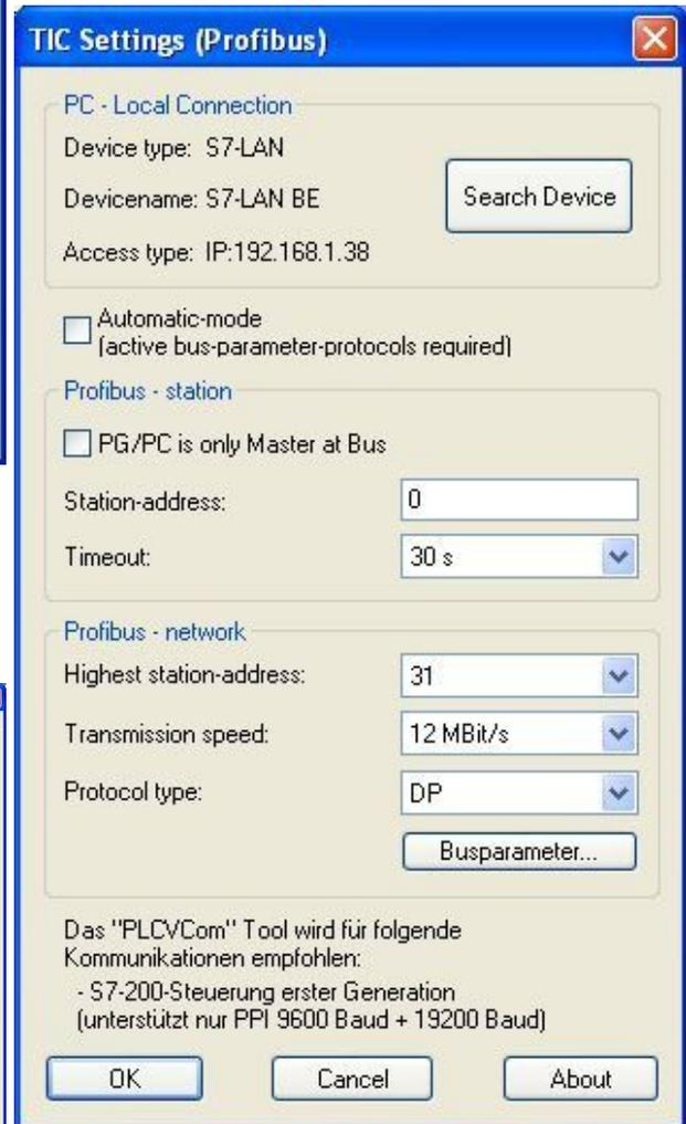
9. If the device-type is not identical with your used device, search for your device with "Search Device". Select the device in the result windows and click on the button "Apply".
