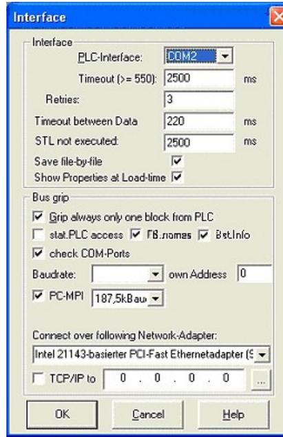
4. Configure the baud rate in the section "Bus access" to "19,2k". Below change the value for PC - MPI to "187,5kBaud".
