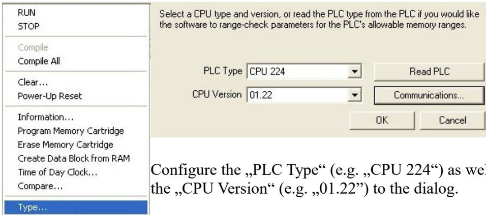
Configure the „PLC Type“ (e.g. „CPU 224“) as well as the „CPU Version“ (e.g. „01.22“) to the dialog.
