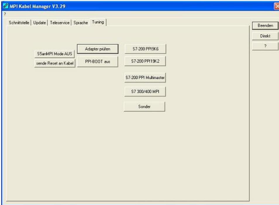
This tab is only used in some special cases. If you press the button „Check Adapter“ the cable is connected and after that the following dialog is displayed:
