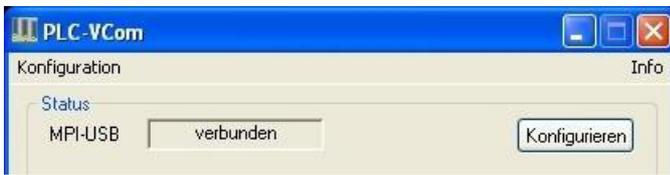
5. In the main window of the PLC-VCOM appears after a successful connection, the type of cable will connect to the computer and the connection status "connected".
