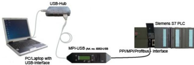
MPI-USB connectivity with the operator terminal
