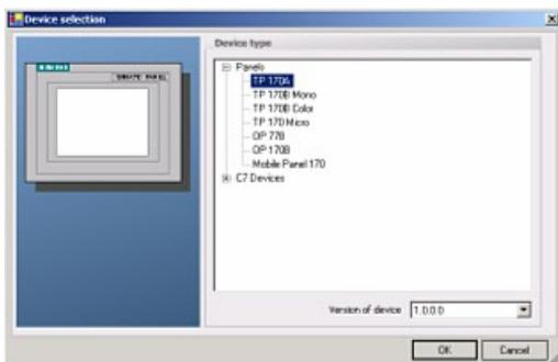
3. In the "Device selection" mark the used operator panel (example: "TP 170A")
