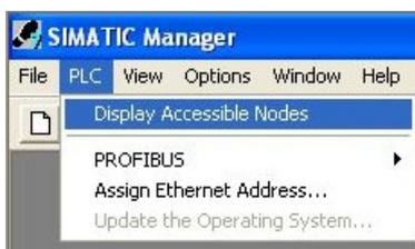
1. Click in the drop - down menu "target system" on "Display Accessible Nodes".
