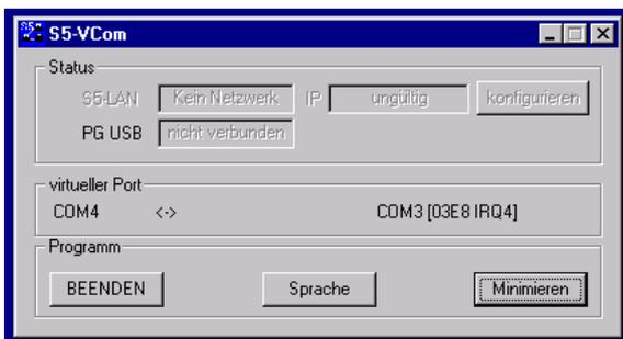
Under the area "Virtual port" on the left side is displayed the COM port that can be used by the Windows software, and on the right side the COM port (IO port) is used by the MSDOS-box.
