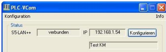
6. In the main window of the PLC VCOMs appears after successfully connecting the cable type, with which the computer connects, the connection status "connected", the IP address and the name of the connected participant.
