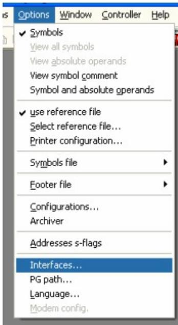
3. A dialog appears. In the section “Interface“ you can configure the “PLC – Interface“ (COM – Port).
