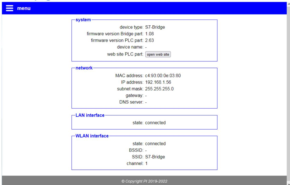
The page “state” is the start page of the device and shows some status information about the device, the current used network addresses and the connection state for LAN and WLAN. Thereby also some information from the integrated S7-LAN or S5-LAN++ are shown.
