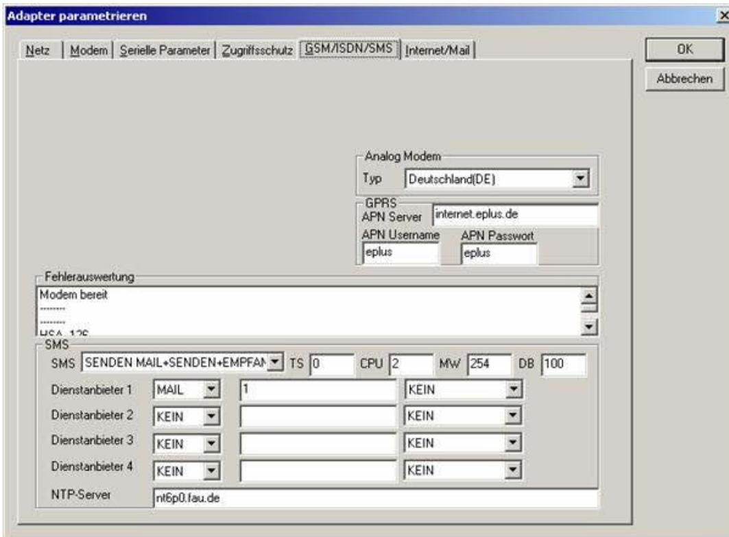
SMS: additionally to the Receiving/sending of SMS and DTMF-processing, the Type "SENDEN MAIL" is usable.
