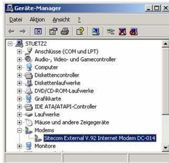
Open the subtree under "Modems" and call the "Properties" of the modem (right mouse button)
