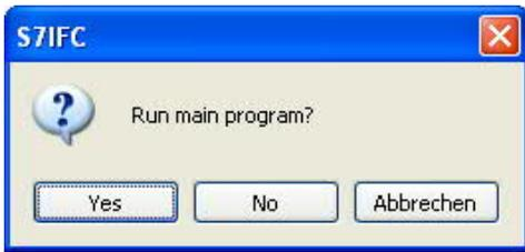
On a click on **Yes** the emergency-loader tries to run the main program of the firmware.
