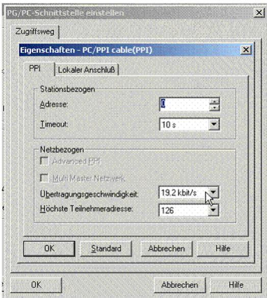
Check under the tab "PPI" the PPI baud rate once again (transmission speed)
