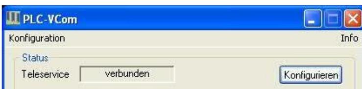
5. In the main window of the PLC VCOMs appears the type of cable will connect to the computer after a successful connection and the connection status "connected".
