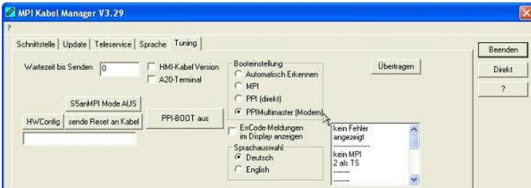
Select under the "Boot Settings", the entry "PPIMultimaster (modem)". Then press the control button "Transfer".
