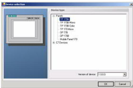
3. In the "Device selection" mark the used operator panel (example: "TP 170A") confirm with "OK".
