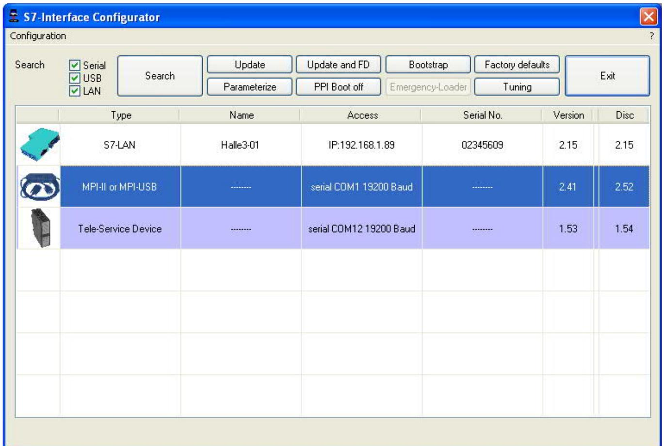
Below the buttons is a list of the found devices. In each line an image, the type of the device, name (if existing), interface, serial number (if possible) and the OS-version of the device is displayed. On the rightmost position the actual OS-version on the harddisk is displayed.
