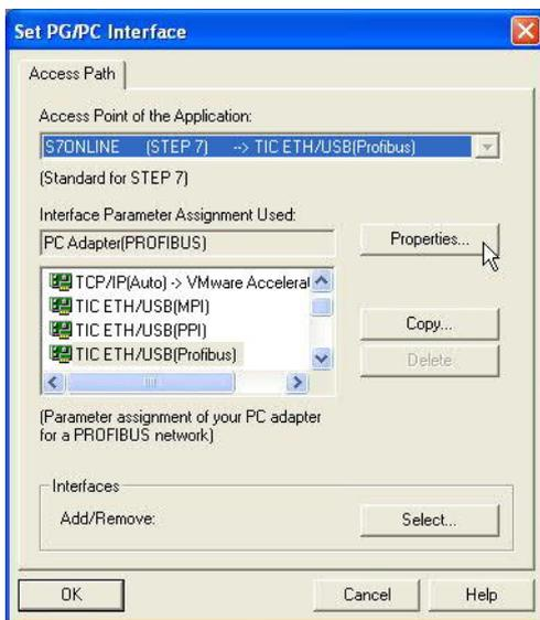
18. If you want to use ProTool/Pro RunTime you can set the "PG/PC Interface" by selecting the "PG/PC Interface" by selecting the entry "DPSONLINE". Therefore you have to select "Access Point of Application" and configure it as described above. The easiest way is to use the S7-LAN/MPI-LAN/MPI-USB-driver which supports USB and LAN products.
