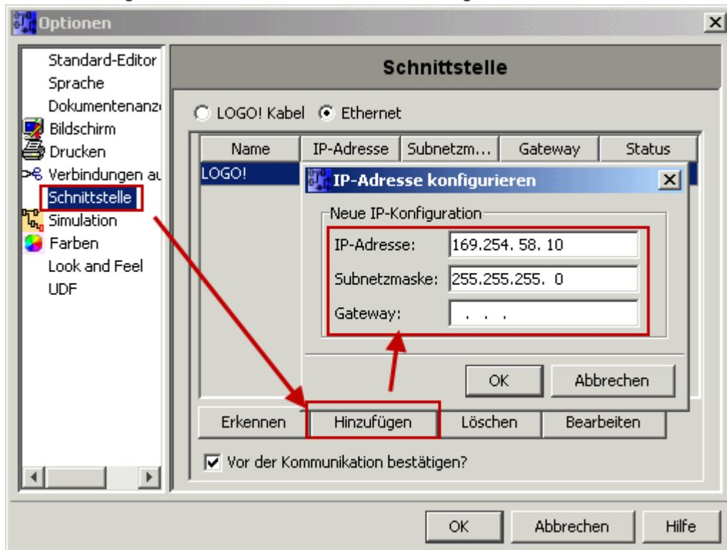
2. Configure PLCs so that connections from an HMI device accepted the Logo!. To do so, go to "Tools- > Ethernet Connections" and then add a new connection.
