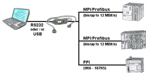
PLC-programming/-communication from the PC "serial" or via "USB" from S7-200/300/400 or modules such as Sinamix, Sinumerik, MicroMaster, drives, converters. PPI up to 187.5 Kbit (PPI + PPI advanced), MPI/Profibus up to 12 Mbit. Compatible with the Siemens driver "PC-adaptor", communication only with 64-bit operating-systems via USB and TIC-driver (limitation of serial communication from Siemens to 32-bit operating-systems).
