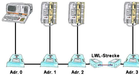
You need for your L1-Bus higher distance like the possible 1200m? You have strong disturbance on your L1-Bus? You need a serial line for higher distances and this galvanic decoupled? No problem, all this points are solved through the LWL-adapter. They are available for artificial and optical fibre, for L1-Bus and RS232.
