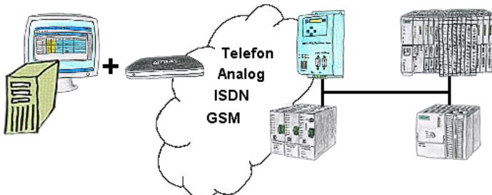
You have to solve a problem in the PLC-program, but the installation is not placed nearby? No problem, start your PG-2000-software with "option teleservice", activate your modem and after selection intra PG-2000-software access to the PLC is possible as if being on-site.
