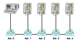
You have to link several S5-PLC's so that in case of need you can respond to all of them without modifying the PLC-program? No problem, connect all PLC's that are in the run with the IBX-Klemme, set up the respective address (1 to 30) at the IBX-Klemme and with the address 0 you will be able to respond to all PLC's via PD-bus-path selection.
