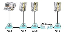
You need for your L1-Bus higher distance like the possible 1200m? You have strong distrubance on your L1-Bus? You need a serial line for higher distances and this galvanic decoupled? No problem, all this points are solved through the LWL-adapter. They are available for artificial and optical fibre, for L1-Bus and RS232.
