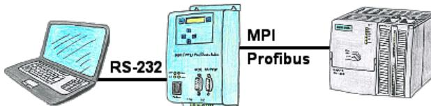
With the MPI/PPI/Profibus-modem you can connect serial to your PC/laptop and then communicate directly with the PLC without a PC-adapter or other S7-programming cables.
