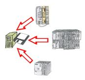
You shortly need a logging of your PLC's operating states respectively are on the way of figuring out a problem and have no datalogger? No problem, connect the PC, start the PG-2000-software with "option datalogger", define relevant variables, appoint timestamp and then the recording starts running immediately. The data will be stored on the fixed disc according to the configuration.
