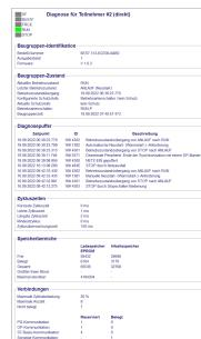
Via the connection-menu and the included bus-device-display, it is possible to display the diagnostics buffer of the respective device without having to open Simatic-Manager or TIA-Portal separately.
