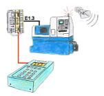
Your installation shows an error and the commissioning engineer isn't available? Connect S5-DIAG with the PLC, enter reason of PLC's malfunction (e.g. O32.5 doesn't come) and the device lists all possibilities why the output has not been set. So you're able to figure out the problem (e.g. safety door not locked) quickly. Finding the cause of the malfunction can be so quick and easy.
