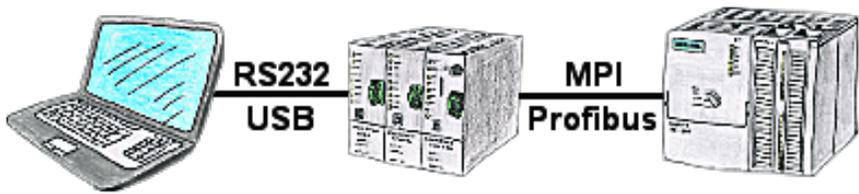
With the TeleService-device you can connect serial or by USB-cable to your PC/laptop and then communicate directly with the control without a PC-adapter or other S7-programming cables.
