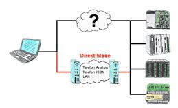
There is an unsupported control or data logger or converter integrated in your installation which protocol is not supported? No problem, the signs that the PC in the office sends will be transferred via telephone line by the Direct-mode, and on-site reproduced by the TP-II. The way back is identical. So in that case there's also a communication to the electronic devices available.
