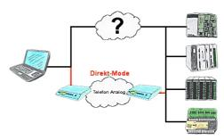
There is an unsupported control or data logger or converter integrated in your installation which protocol is not supported? No problem, the signs that the PC in the office sends will be transferred via telephone line by the Direct-mode , and on-site reproduced by the TP/TB. The way back is identical. So in that case there's also a communication to the electronic devices available.
