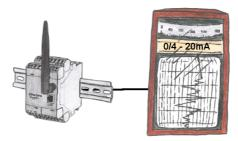
By connecting a line-recorder to the EtherSens-device anyone without network-knowledge can visually capture and further process the log.
