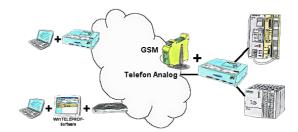
Access to the connected PLC takes place by coupling via Analogue-, ISDN- (only with AB-adapter) and GSM-(only with external GSM-modem)-line.
