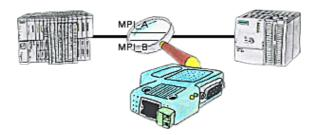
The S7-LAN can also be used for controlling/checking the MPI/Profibus. It will be plugged on the Bus so that you can take a look at the status of the busses via software on PC, for example the numbers of parity errors.
