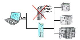
Do you have a PLC without CP343-1 or CP443-1 and a TP-II as remote maintenance device? Then activate the CP-mode of the TP-II and your visualisation goes directly ONLINE via the LAN of the TP-II.
