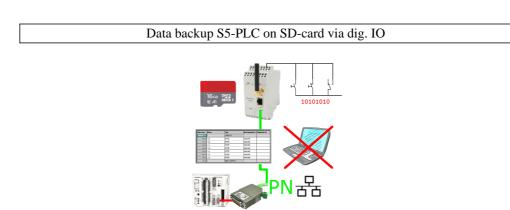
Via digital input triggered DB-backup/-restore without additional PC via PG-socket and Ethernet to SD-card
