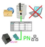
S7-PLC triggered DB-backup/-restore without additional PC via MPI/Profibus on FTP-server
