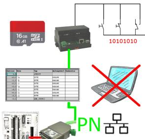
Via digital input triggered DB-backup/-restore without additional PC via PG-socket and Ethernet to SD-card
