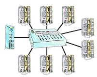
You have many PLC and you want to programm them central on one place? No problem, you have to connect them all to the KOR/MUX-Tele-Switch, connect it with the TP-II and after telephone connect you will be able with the PD-bus-selection of your Step5-software to go ONLINE. Of course the MOR/MUX-Tele-Switch is cascadable, so you can connect up to 30 PLCs to the devices.
