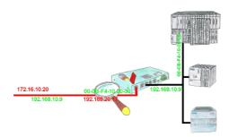
You have in your facility machines from different manufacturers and no one does get access to the controls of the other? No problem, with the S7-firewall you can filter who can ever communicate with the control network and which user with which end users. This is done through the IP address and MAC address.
