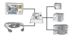
Do you have a single control with panel in use and have to accomplish a little modification in the control program? No problem, plug the T-Connector on the PLC, the panel and PC to the device and then both participants can work with the PLC without annoying bus-cable tapering and interconnections.
