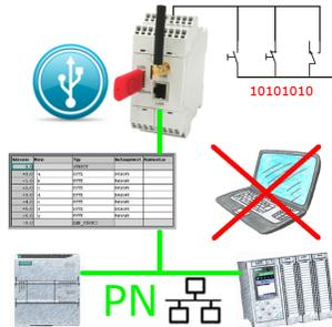
Via digital input triggered DB-backup/-restore without additional PC via PN-port to USB-stick
