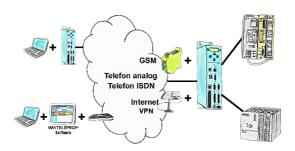
Access to the connected PLC takes place by coupling via Analogue-, ISDN-, mixed Analogue-ISDN-, GSM-, UMTS-line and also via Internet with and without VPN-security.
