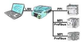
S7-PLC with PPI, MPI, Profibus connection, but data should be read/written via network?
